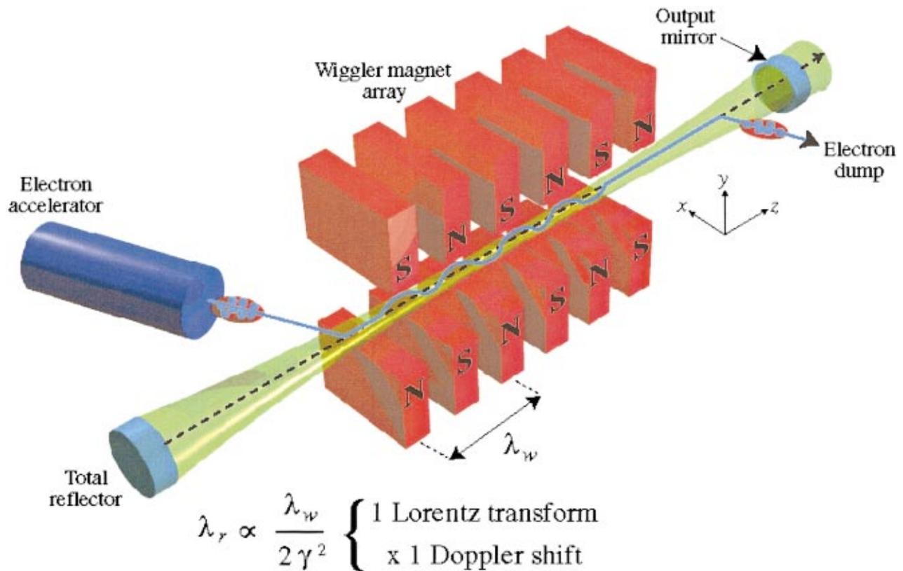
FIG. 1. Components of a free-electron-laser oscillator [Color].
