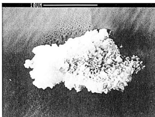
**Figure 37.** SEM photomicrograph of a field emitting microparticle found by temperature mapping and subsequent dissection of a single-cell 3 GHz cavity. EDX analysis shows that the particle contains titanium, carbon, oxygen, sodium, indium, aluminium and silicon. Note the very rough surface of the particle. Such protrusions cause geometric field enhancement [56].
