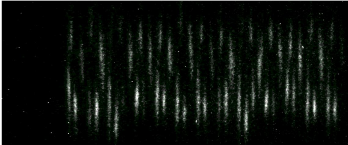
Minor-axis projection showing injected charge arriving on the 13th of 80 consecutive turns.
