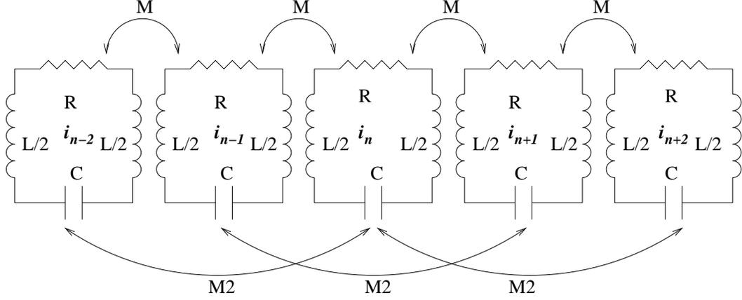
Figure 7: Equivalent circuit for an infinitely long magnetically coupled linac structure. This linac is a single periodic structure meaning that every cavity cell is identical.
