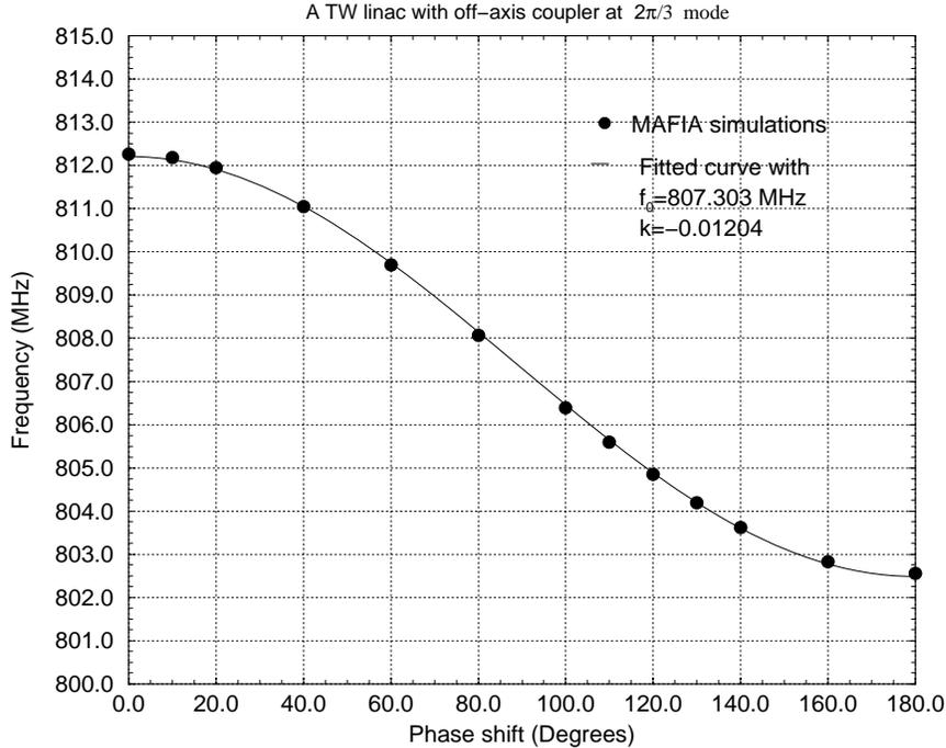
Figure 2: Dispersion relation of a  $\frac{2\pi}{3}$  off axis coupled traveling wave structure.
