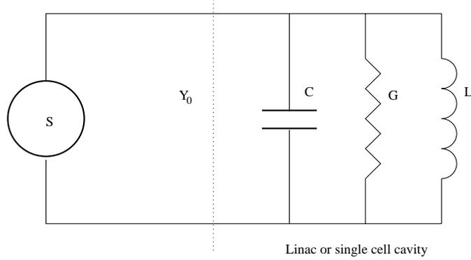
Figure 8: Equivalent circuit for a linac or a single cell cavity coupling to a RF source.
