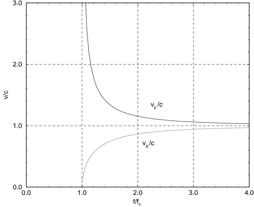
Figure 1: Frequency characteristics of phase and group velocity in waveguides
