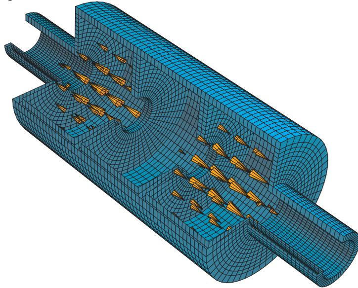
Figure 5: Electric field distribution of the  $\frac{\pi}{2}$  mode of the USPAS linac. The calculated resonant frequency of this mode is 2.605 GHz.
