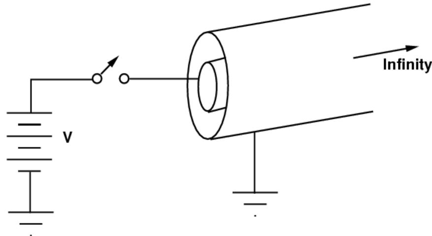
Take an infinitely long coaxial cable and suddenly apply a voltage  $V$  to it. A current  $I$  will flow, determined by the capacitance and inductance of the cable. The ratio of the voltage  $V$  to the current  $I$  is the **characteristic (or surge) line impedance  $Z$** .
