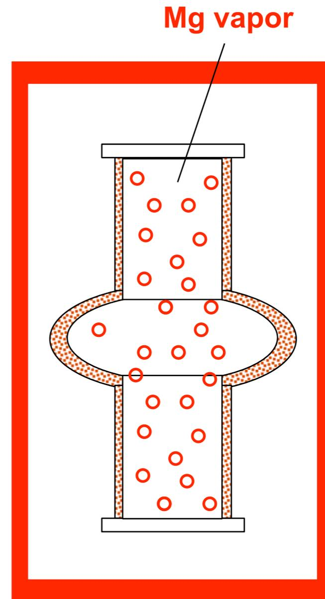
Reacting with Mg to form  $MgB_2$  at  $\sim 850-900^\circ C$  in Mg vapor
