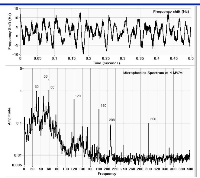
Time domain and frequency domain plots of the background microphonics for a 5-cell CEBAF cavity located in the CEBAF accelerator.
