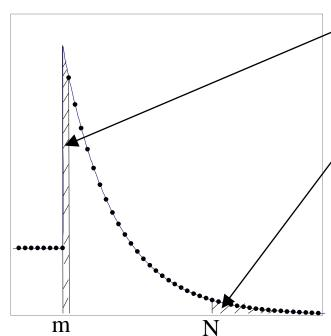
$(\Delta P_{emitted})_m \Delta t$  is due to the jitter in the start of the integration and the peak of the emitted power transient
