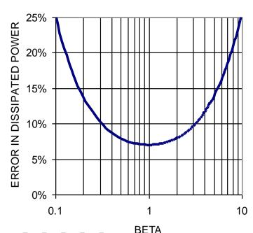
As was stated earlier,  $\beta$  is a measure of the magnitude of the reflected power as compared to incident power. At  $\beta = 1$  the error in the dissipated power, as measured using the RF signals, is minimized and approximately the value of the error in the incident power. As  $\beta$  gets much above 8 and much below 0.15 the errors in dissipated power, and subsequently calculated values of  $Q_0$  start to become excessive.
