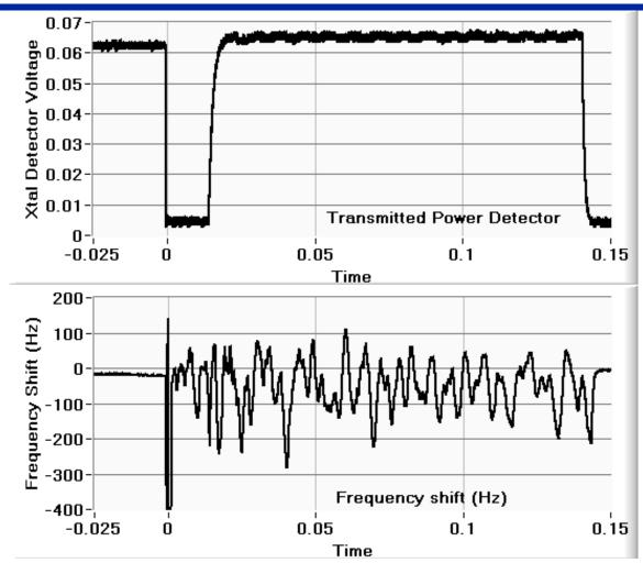
Vibrational modes excited by the sudden loss of cavity gradient due to a window discharge on the cavity side of a cold window in the same cavity as the previous slide.
