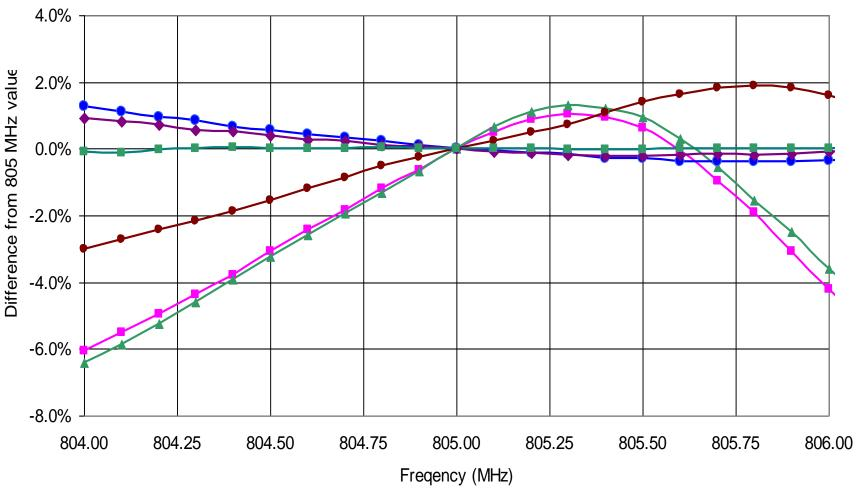
Difference between RF readings calibrated at 805 MHz and those taken at nearby frequencies for several different signal paths. The paths with smaller errors had attenuators distributed throughout the signal path.
