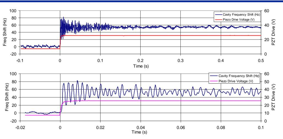
Step response of a cavity excited by a by a 50 Hz step in the piezo tuner controls. The total range of this tuner was 550 Hz.
