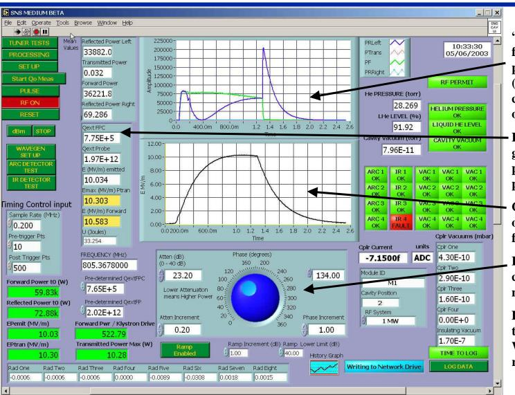
"Real time" gradient and forward and reflected power waveforms shown (supplemented with crystal detectors and an oscilloscope)
