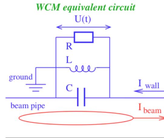
Schematics of a wall current monitor and its equivalent circuit [1]
