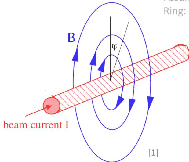
$$\text{Line current field: } \vec{B} = \mu \cdot \frac{I_{beam}}{2\pi r} \vec{a}_\varphi$$
