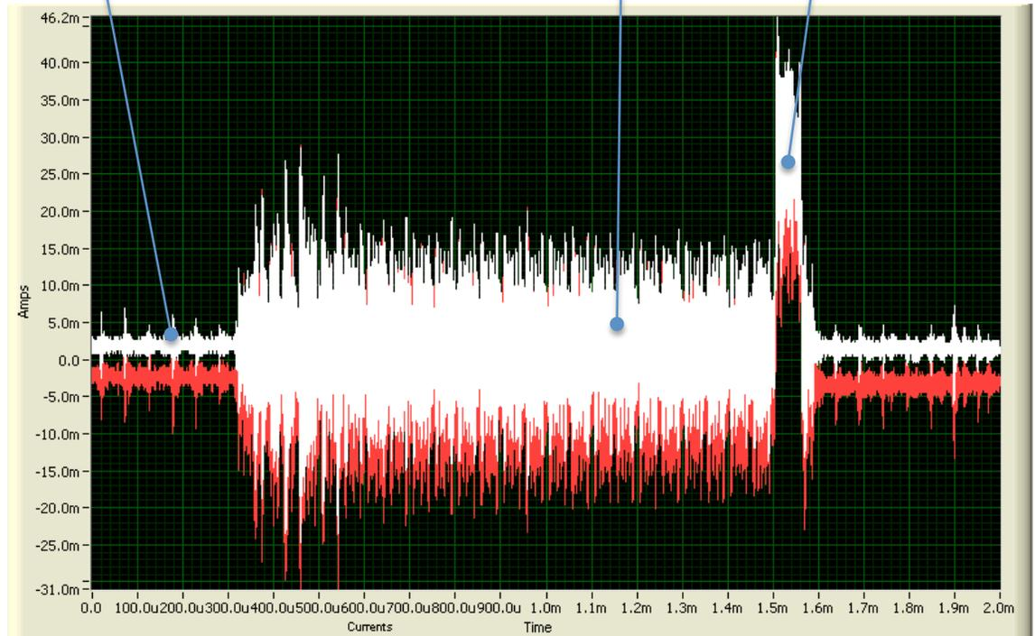
Noise of DTL current transformer (inside cavity, single ended)
