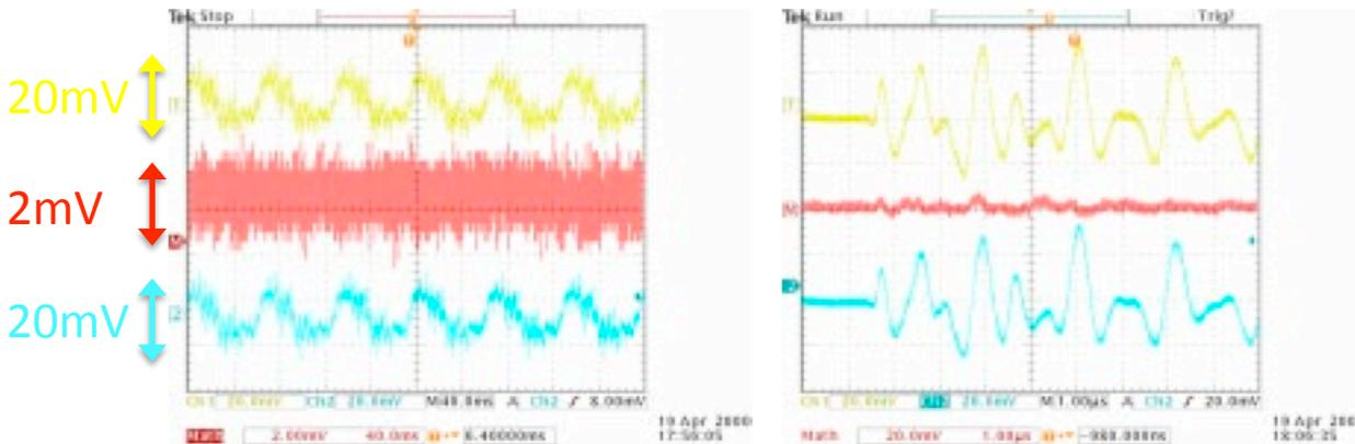
Differential noise on long twinax with far end shield grounded. Left: top and bottom, noise on either center conductor into 50 ohms (each 20mV/div); center, difference (2mV/div); (most of residual signal due to digital scope subtraction). Right: same signals faster time scale (each 20mV/div and 1uS/div). From [2] Webber.
