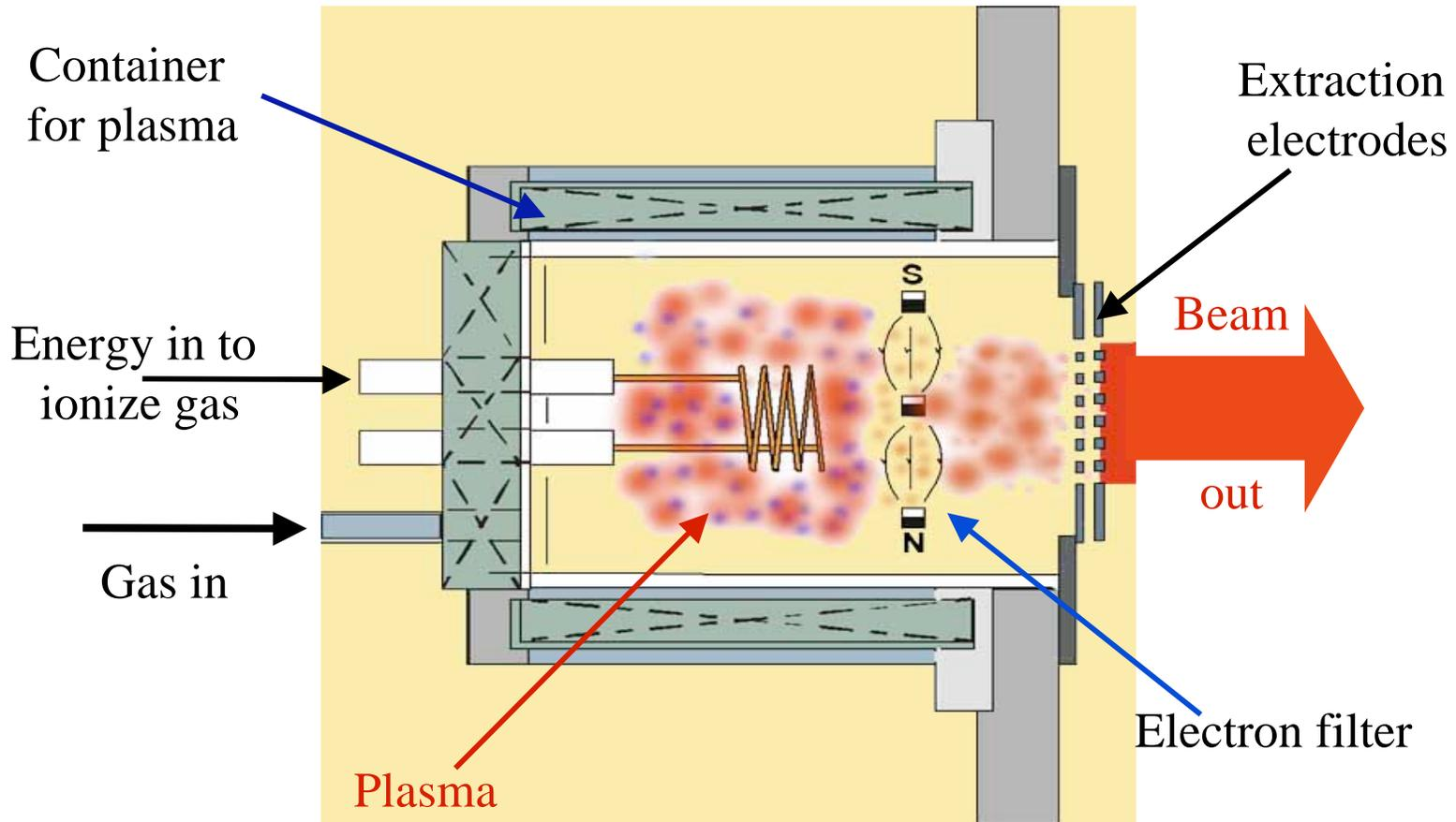
*Electron beams can also be used to ionize the gas or sputter ions from a solid*
