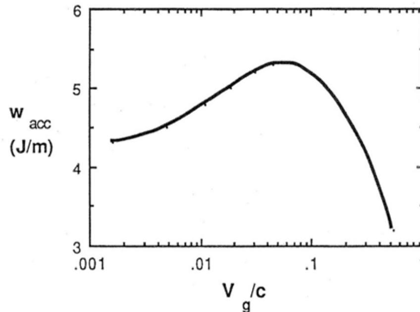
$$s_t = \frac{E_{peak}^2}{w_{acc}} = 5.7 \times 10^{14} \text{ V/mC} \left( \frac{10\text{mm}}{a} \right)^2 \beta_g^{0.4}$$
