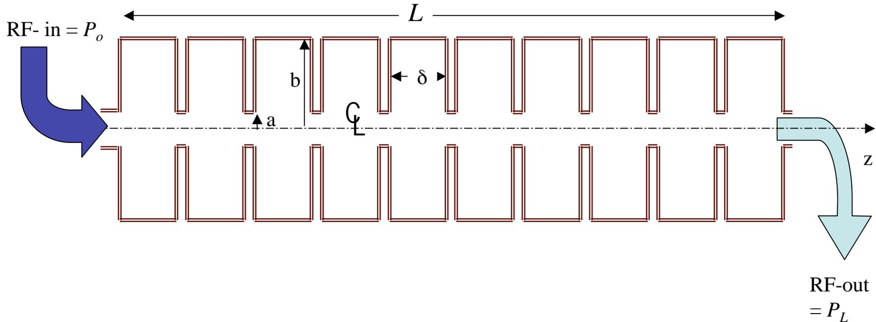
In a structure with a constant geometry, the inductance & capacitance per unit length are constant
