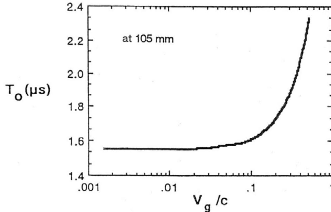
$$T_o = 1.45 \mu\text{s} \left( 1 + 1.29 \beta_g^{3/2} \right) \left( \frac{\lambda}{105 \text{ mm}} \right)^{3/2}$$
