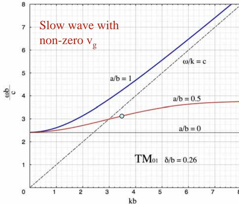
Small changes in  $a$  lead to large reduction in  $v_g$
