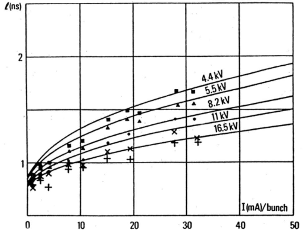
Fig. 13. Bunch length measurements on ACO.
