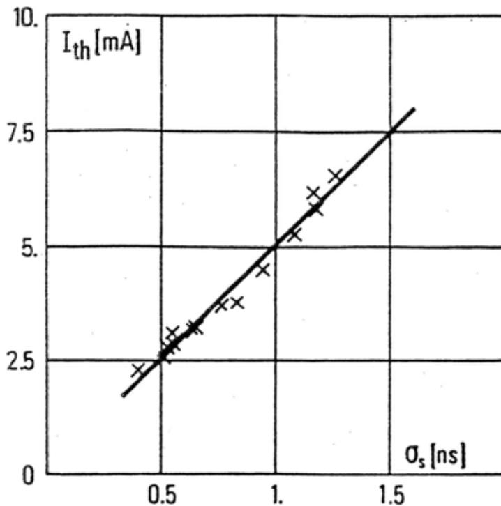
Fig. 9. Transverse instability threshold vs bunch length measured on ACO.
