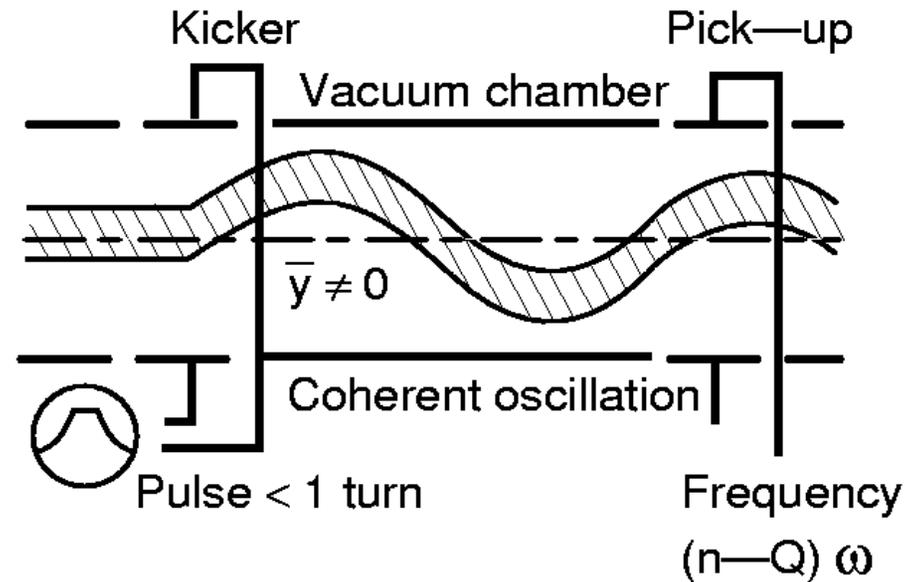
Center of mass moves with a betatron oscillation
