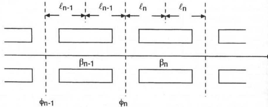
Figure 6.2. Accelerating cells for describing the longitudinal motion.
