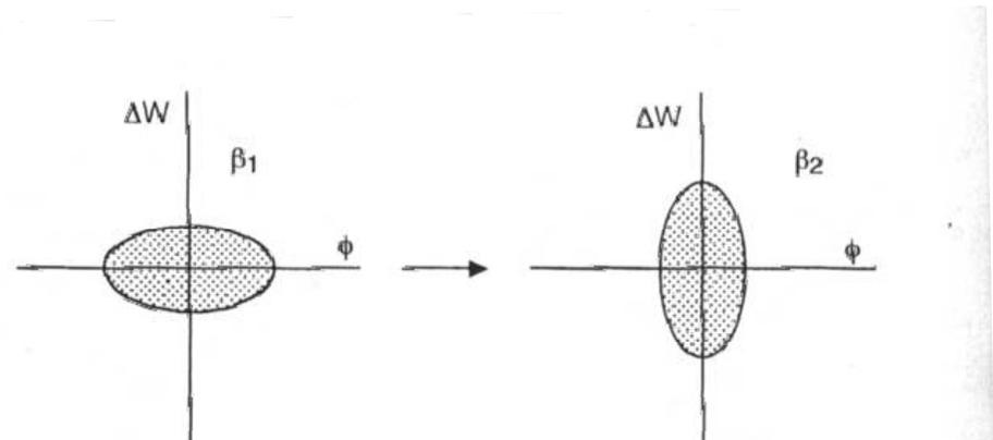
Figure 6.8. Phase damping of a longitudinal beam ellipse caused by acceleration. The phase width of the beam decreases and the energy width increases while the total area remains constant.
