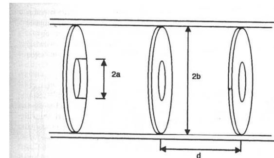
Figure 3.14 Iris (disk)-loaded traveling-wave structure.
