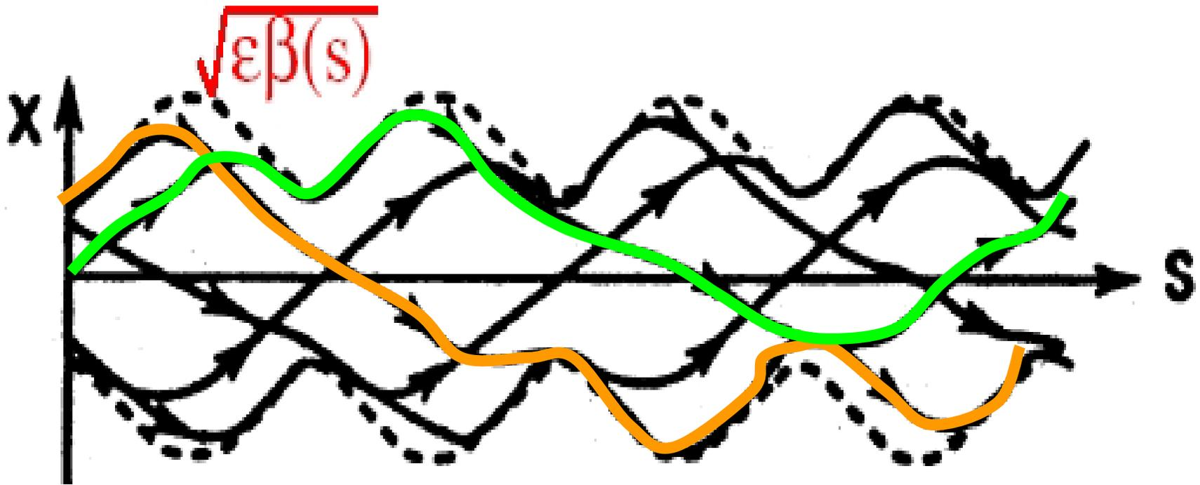
As the beam follows its trajectory, different particles occupy the beam envelope. In reality, we don't much care which particles are on the envelope, **we care about the shape and extent of the envelope itself.**
