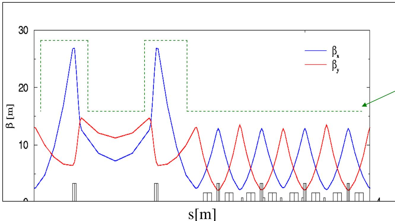
Beam pipe aperture scales with beta function.
