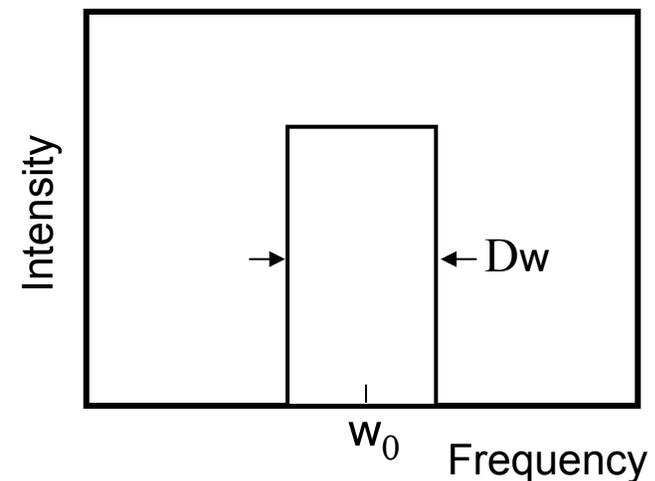
The Michelson interferometer output—the interferogram—Fourier transforms to the spectrum.
