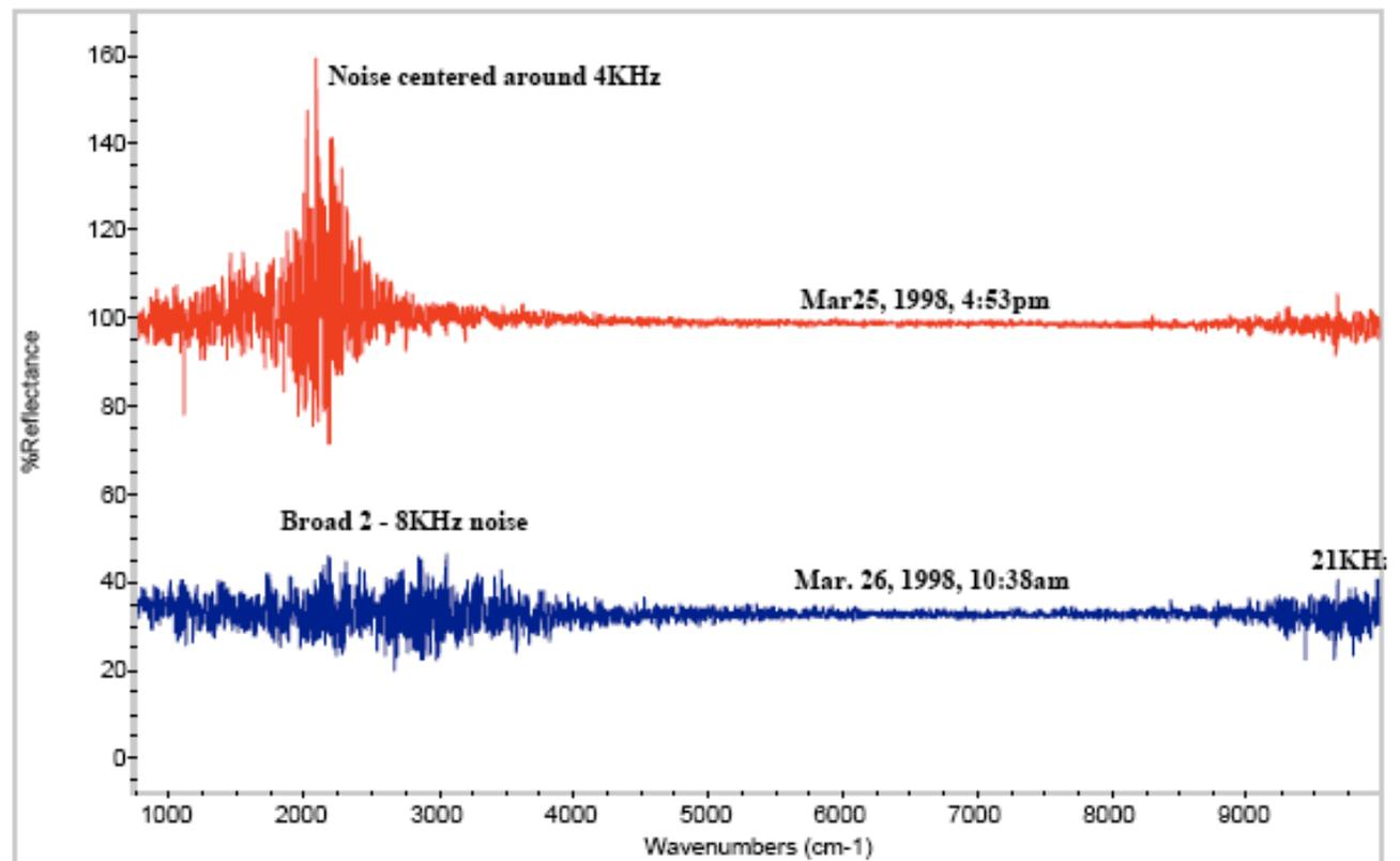
Figure 1. FTIR Spectra showing extra noise in the 2 – 8 kHz frequency regime.
