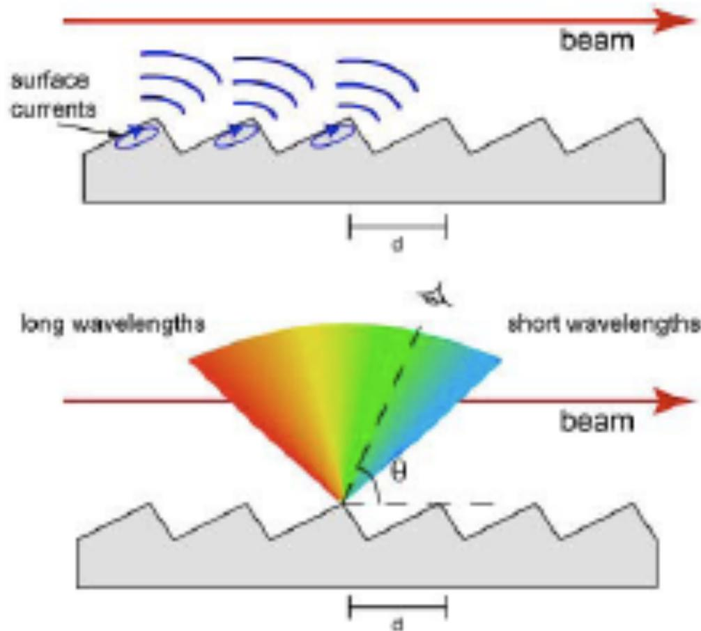
Smith-Purcell radiation is interference of multiple diffraction radiators
