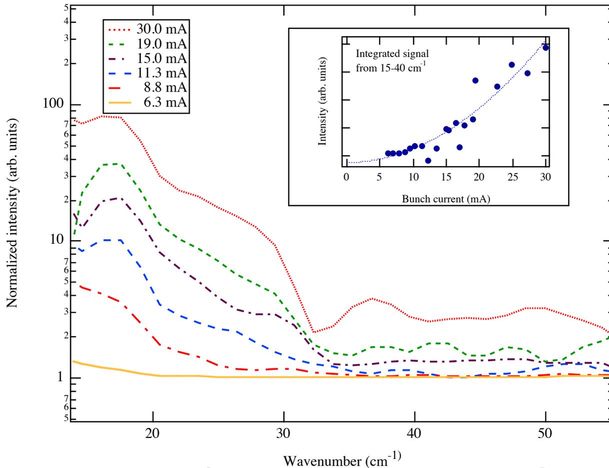
Signal during microbunching “bursting” instability in the ALS.
