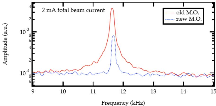
Noise identified as synchrotron motion (Robinson mode). New master oscillator reduces motion and solves problem.
