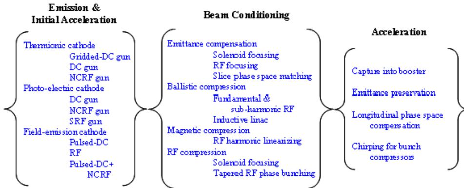
FIGURE 7. The basic parts of the electron injector.
