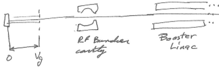
FIGURE 3. An early injector for bunching the beam into the phase space acceptance of the booster linac. In this approach, the DC beam from a thermionic gun is first energy modulated by the buncher cavity which ballistically compresses electrons over less than 180 degS at the buncher cavity.
