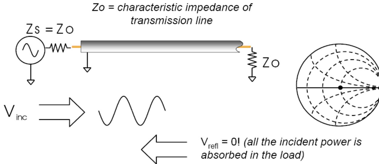
For reflection, a transmission line terminated in  $Z_0$  behaves like an infinitely long transmission line
