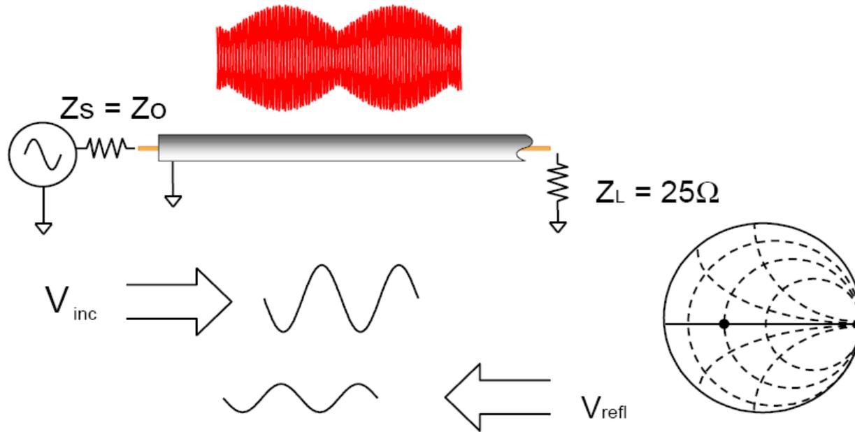
Standing wave pattern does not go to zero as with short or open
