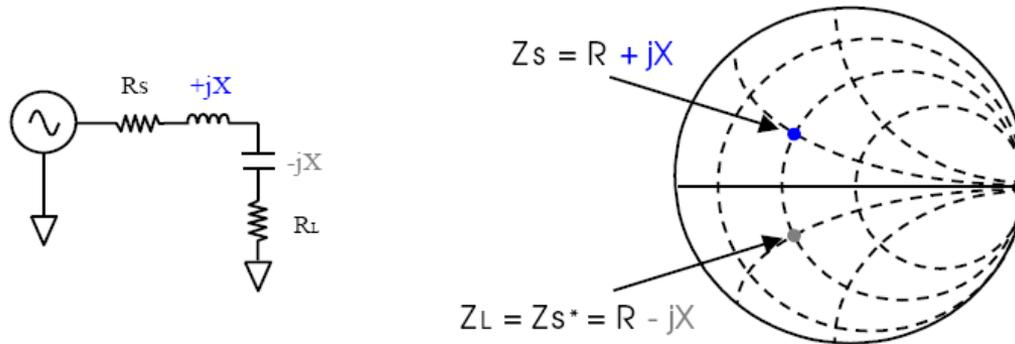
At high frequencies, maximum power transfer occurs when  $R_S = R_L = Z_0$
