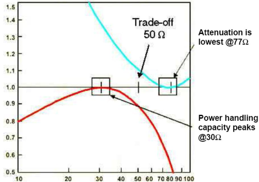
Characteristic impedance for coaxial airlines ( $\Omega$ )
