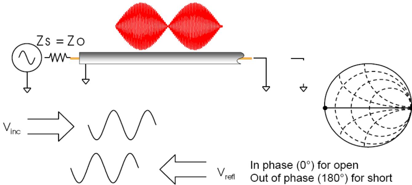
For reflection, a transmission line terminated in a short or open reflects all power back to source
