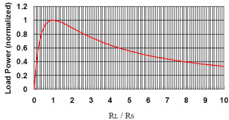
*Maximum power is transferred when  $R_L = R_S$*
