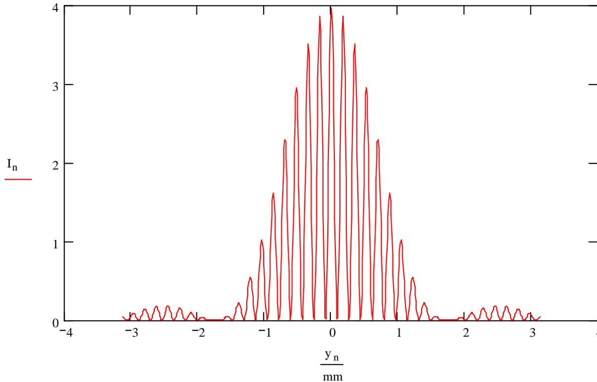
Fringe pattern of a monochromatic point source at 450 nm, using parameters for the PEP-II HER interferometer at SLAC.  $A_1 = A_2 = 1$ ,  $d = 5$  mm,  $a = 0.5$  mm.
