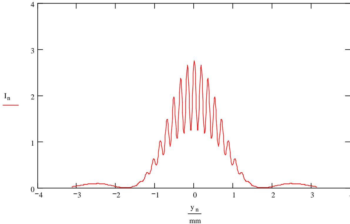
Fringe pattern using a Gaussian bandpass filter with a full width at half maximum (FWHM) of  $\Delta\lambda = 30$  nm.
