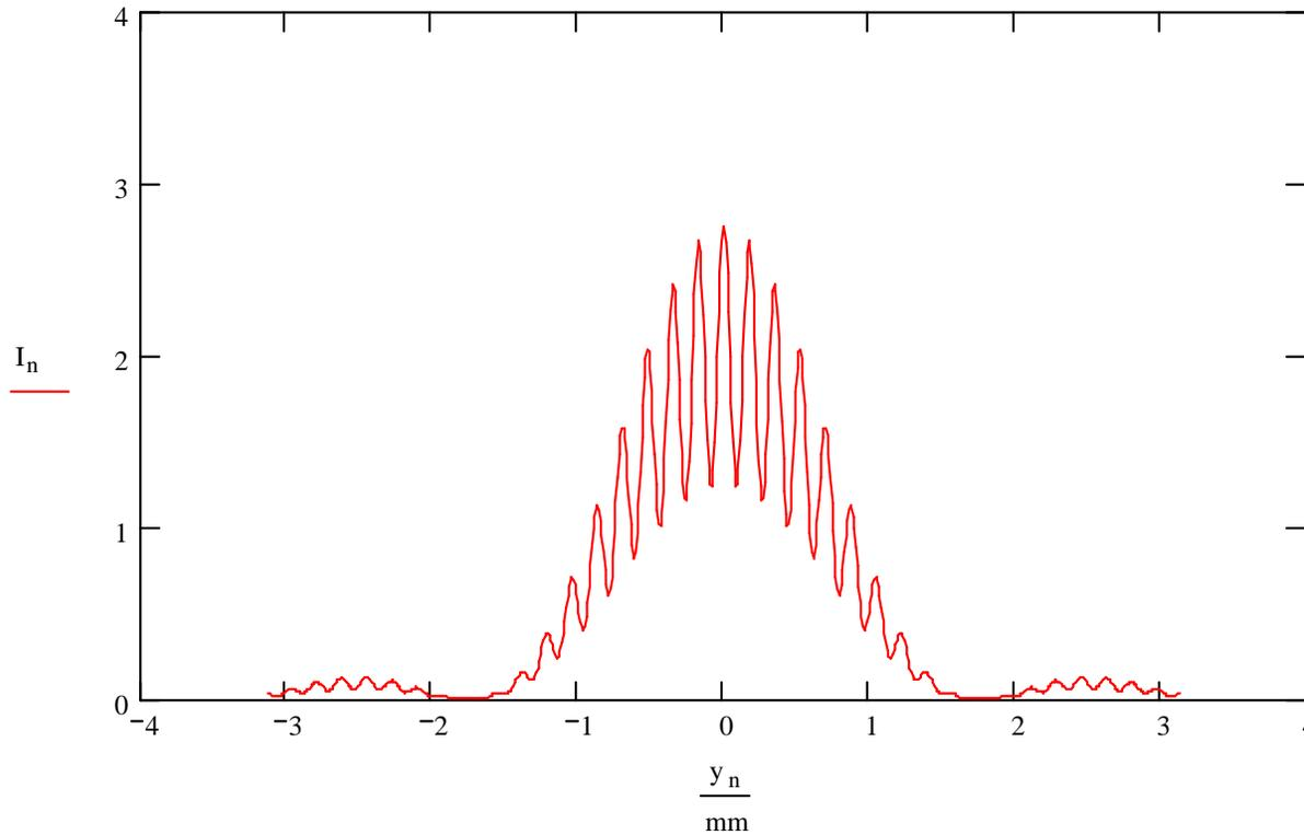
Fringe pattern of an extended source, with  $\sigma_0=0.2$  mm
