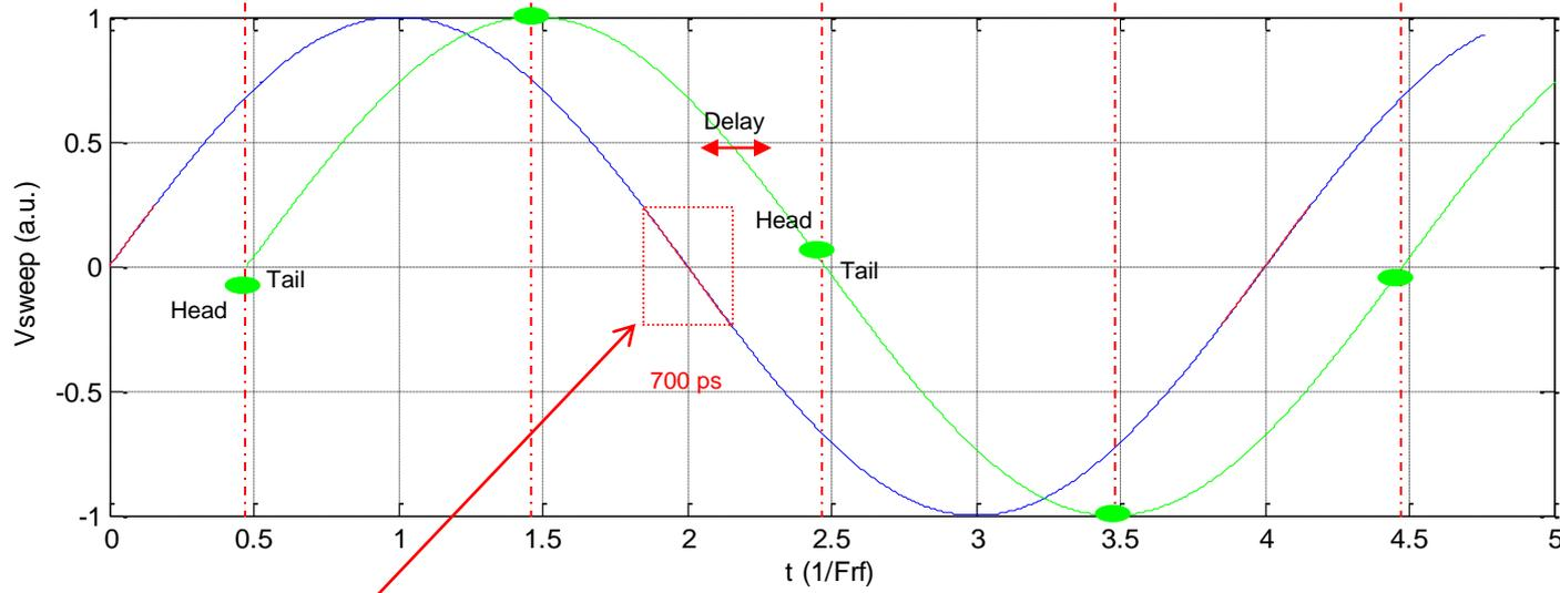
Streak camera sweeping signal, RF/4, delay adjustable
