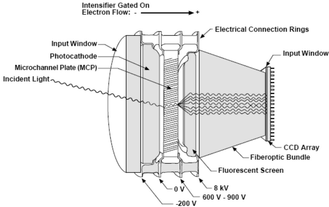
Figure 2. Major Components of the Intensifier-CCD
