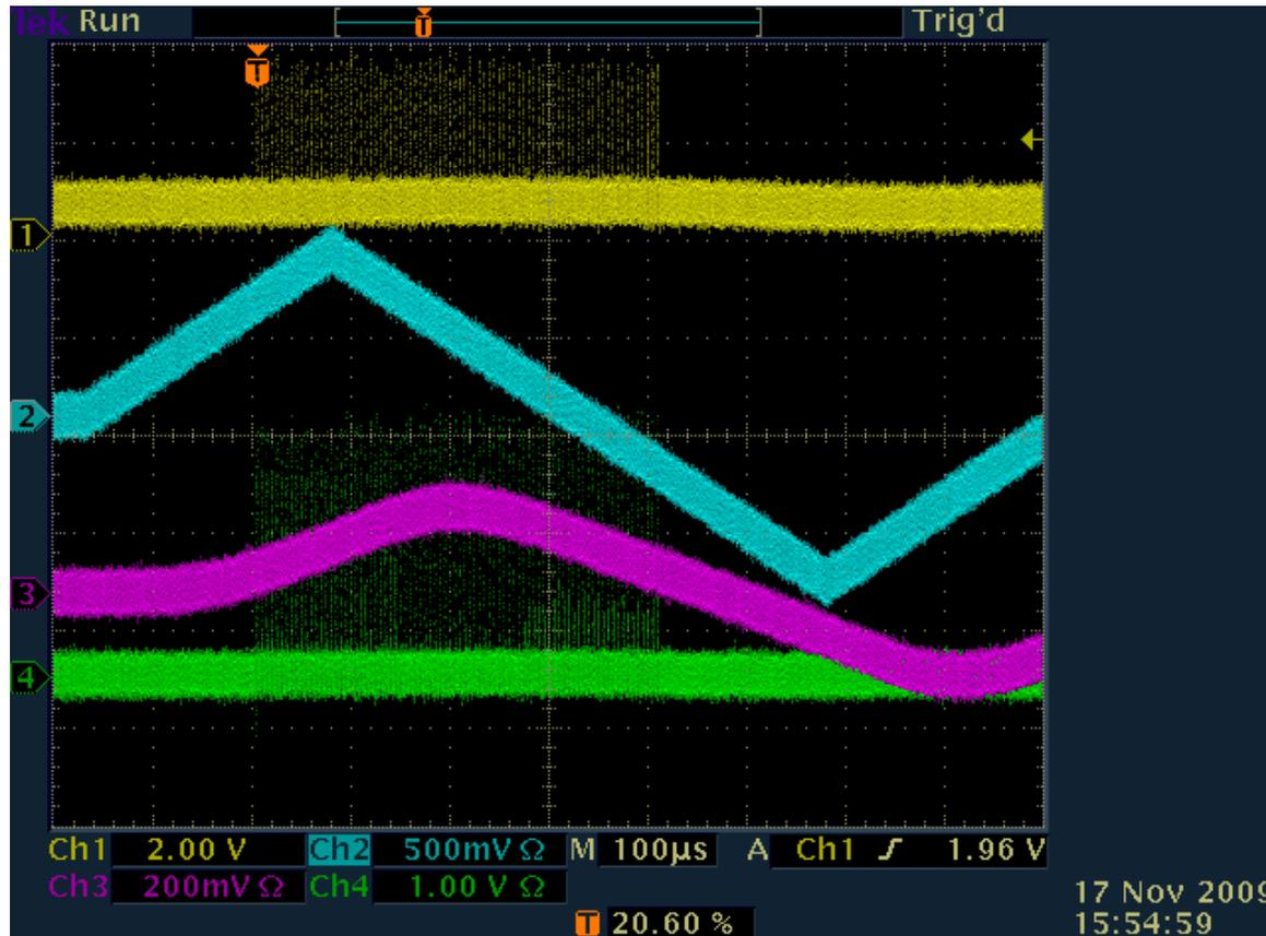
CH1 LED drive signal, 200kHz repetition rate, 15ns minimum
