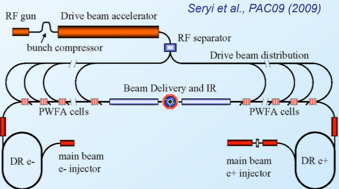
Figure 1: Concept for a multi-stage PWFA-based Linear Collider.
