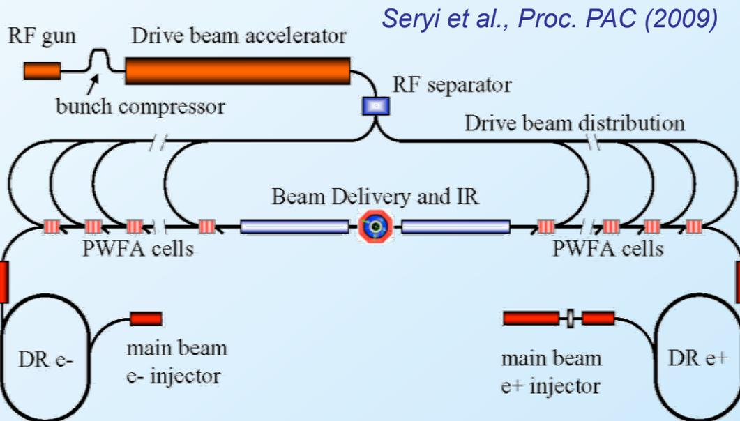
Figure 1: Concept for a multi-stage PWFA-based Linear Collider.
