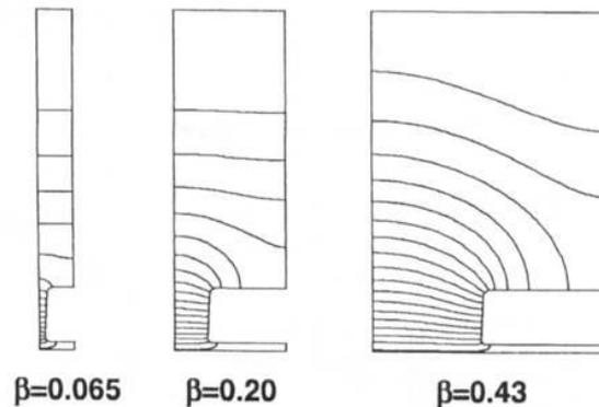
Figure 4.9 Electric-field lines shown in one quarter of the projections of three DTL cells as calculated by the program SUPERFISH (courtesy of J. H. Billen).
