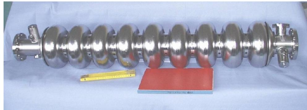
Superconducting RF cavity for ILC
