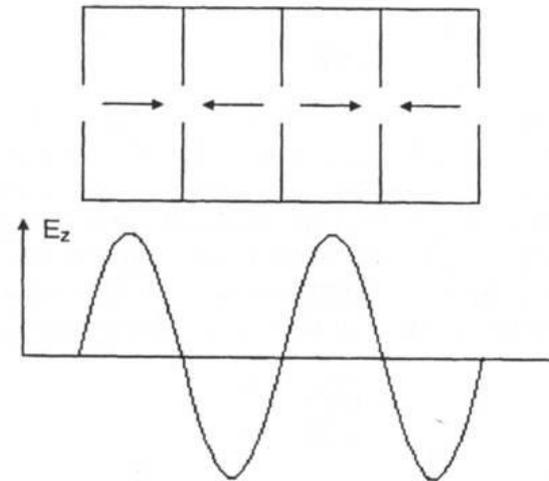
Figure 2.3 Axial electric-field distribution showing the effect of the  $\pi$ -mode boundary conditions, which causes the field to cross the axis at the boundaries of each cell.
