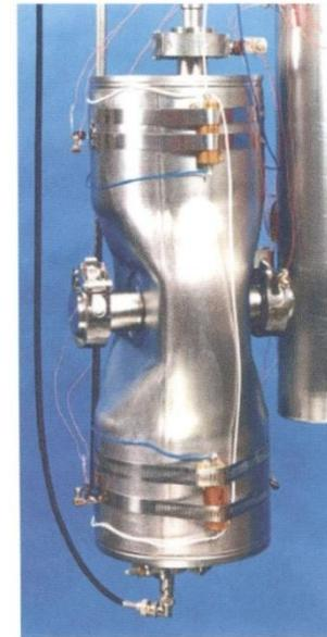
**Figure 4.26** 350-MHz  $\beta = 0.12$  coaxial half-wave resonator with a single loading element (courtesy of J. R. Delayen, Ref. 33).
