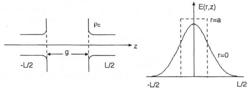
Figure 2.1 Gap geometry and field distribution.
