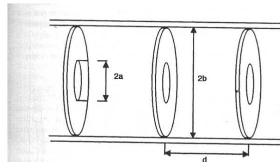
Figure 3.14 Iris (disk)-loaded traveling-wave structure.
