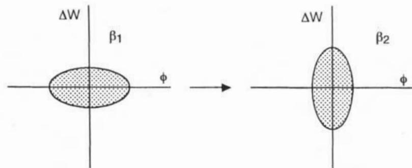
**Figure 6.8.** Phase damping of a longitudinal beam ellipse caused by acceleration. The phase width of the beam decreases and the energy width increases while the total area remains constant.
