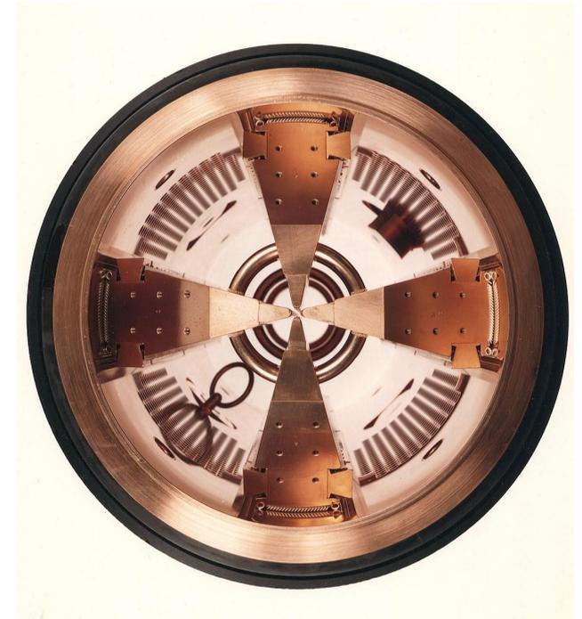
Many laboratories have adopted the RFQ as a front end accelerator for injectors for synchrotrons. The RFQ has almost completely replaced large 750 kV air-insulated Cockcroft-Walton accelerators (except at FNAL and LANSCE). RFQs have a smaller footprint and a lower cost of maintenance than CW pre-accelerators.
