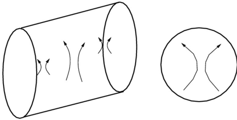
The TE field in a pillbox cavity must go to zero at the ends, due to the boundary condition that the E-field has no component parallel to a conducting surface.
