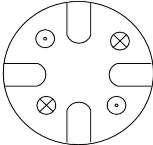
The magnetic field in the  $TE_{210}$  mode alternates in adjacent quadrants. At the ends, the magnetic field passes around the vane cutbacks.
