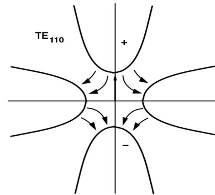
The vanes concentrate the electric field on axis. The  $TE_{110}$  mode is a deflecting mode
