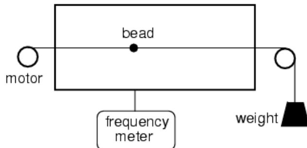
The beam is usually drawn through by a motor drive, and the measured frequency shift recorded on a computer.
