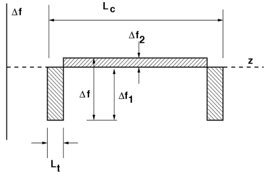
This is the change of overall frequency of the cavity due to the tuner offset. To satisfy
