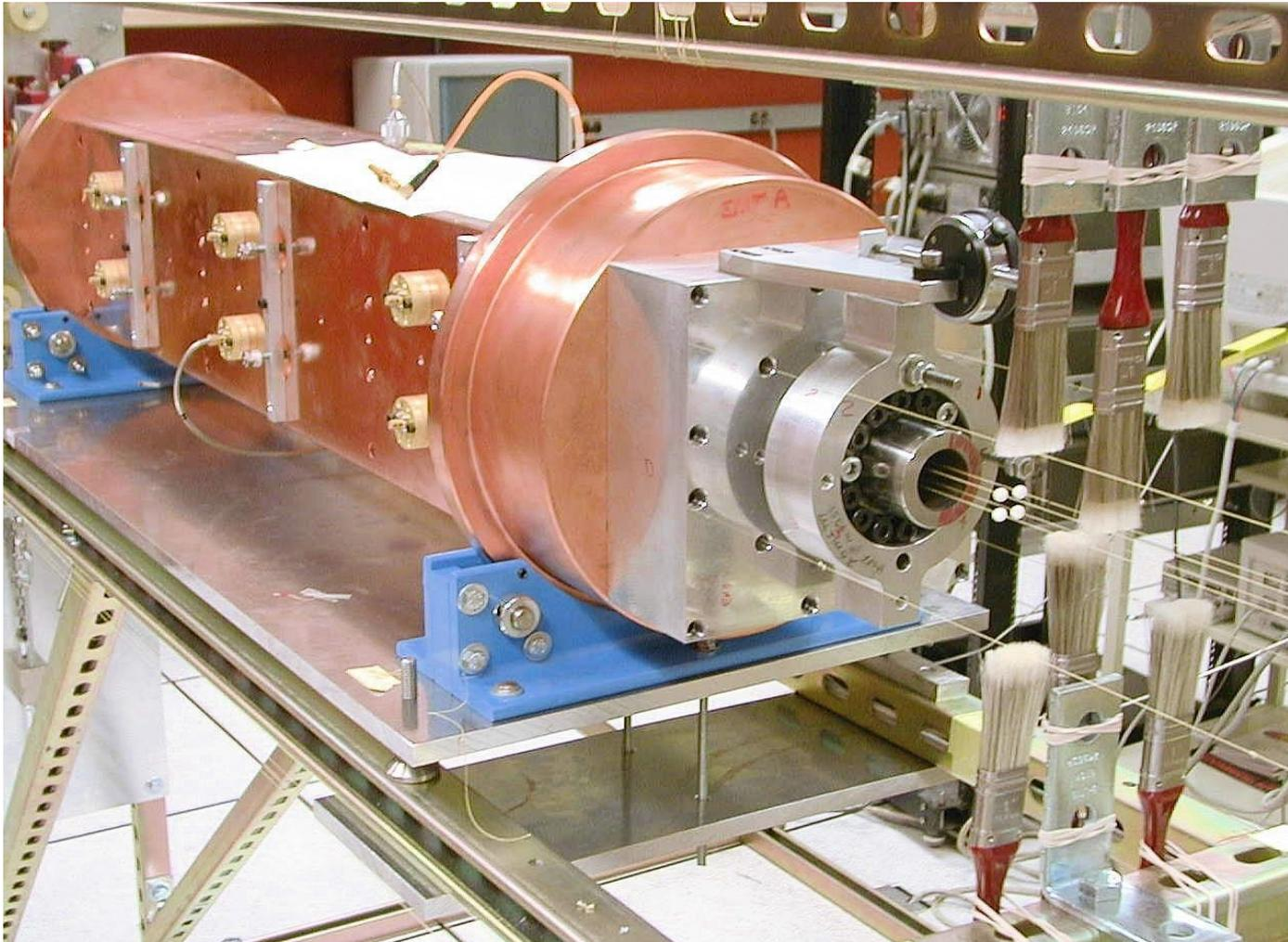
Here, four beads are pulled independently through the four quadrants of the RFQ near the vane tips near maximum E-field.
