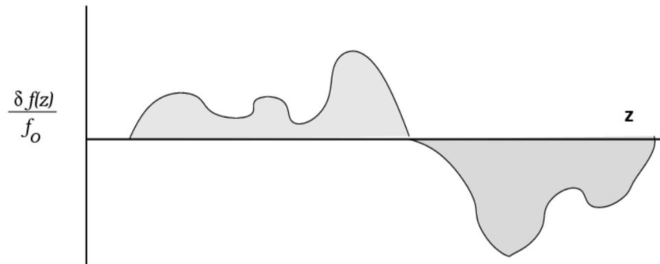
The frequency shift of the cavity due to perturbations is  $\Delta f = \frac{1}{L_{cav}} \int \delta f(z) dz$
