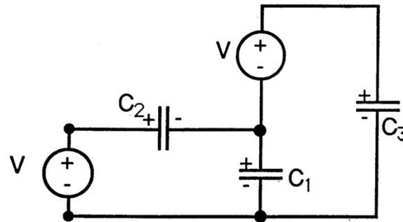
$C_1$ : stage to ground capacitance
