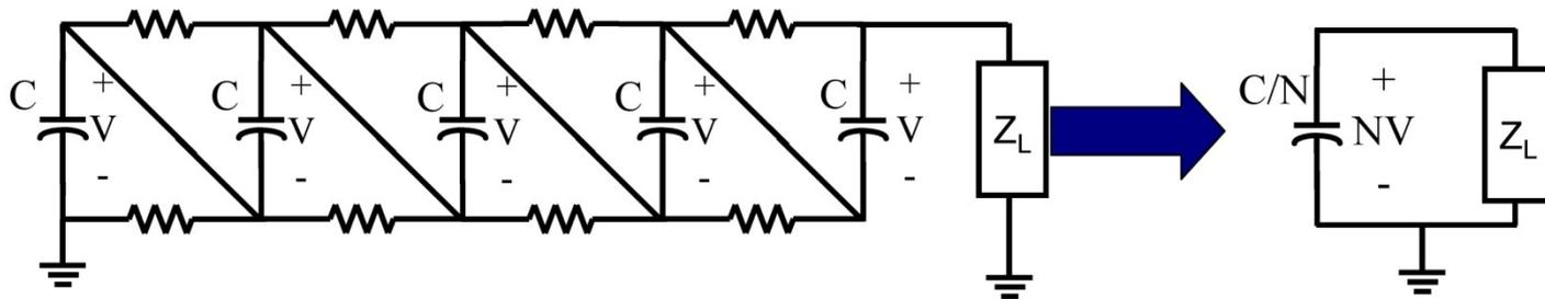
Erected stage configuration of a 5-stage Marx bank
