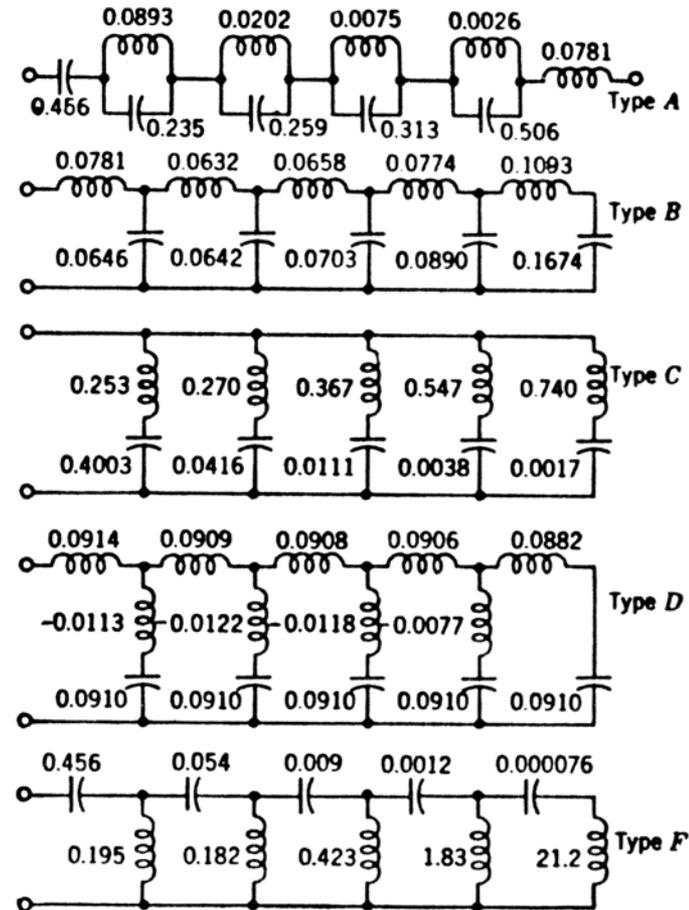
FIG. 6-22.—Equivalent forms for five-section Guillemain voltage-fed network. Multiply the values of the inductances by  $Z_N \tau$  and the values of the capacitances by  $\tau / Z_N$ . The inductances are in henrys and the capacitances in farads if pulse duration  $\tau$  is expressed in seconds and network impedance  $Z_N$  in ohms.
