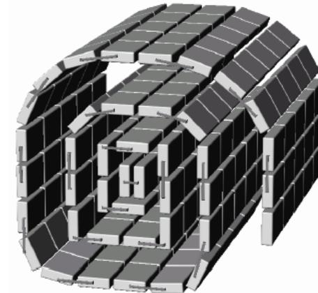
*Solid model of the 500 kV hard switch – note the spiral wrap of the series string of switch modules to reduce effective parasitic capacitance. The output (pulsed) end of the modulator is on the axis, and the input (DC) end is on the outer surface.*
