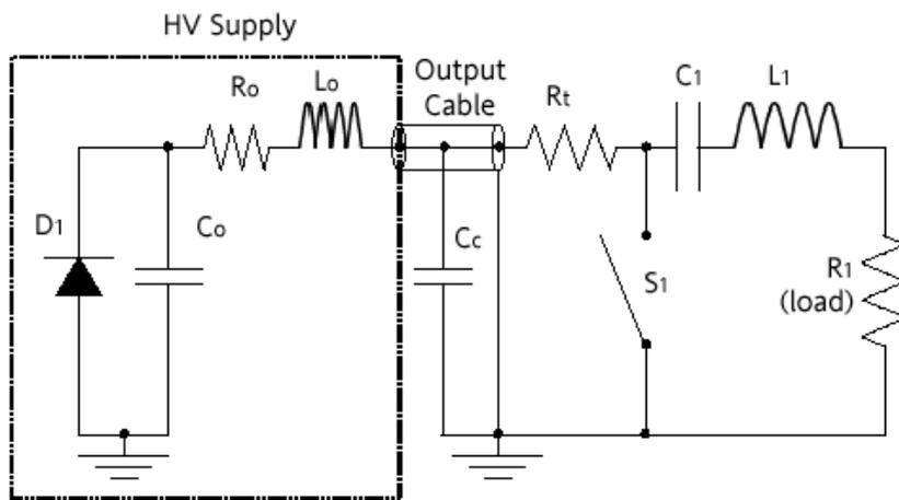
$R_t$  terminates the output cable and prevents the voltage reversal from the closing of switch  $S_1$  from appearing across  $D_1$ .  $R_o$  is the internal resistance of the power supply and is usually on the order of a few ohms.  $C_o$  is the internal power supplies internal capacitance and may only be a few hundred pF.
