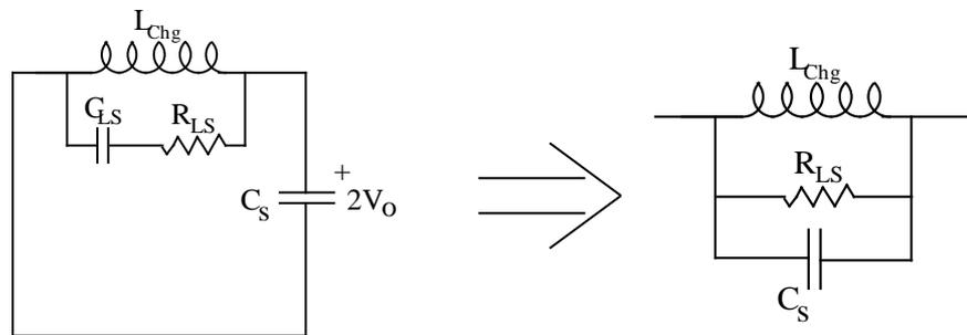
Equivalent circuit with snubber across inductor
