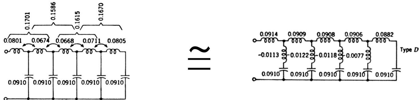
The negative inductance that are seen in the Type D PFN represent the mutual inductance between adjacent inductors and may be realized in physical form by winding coils on a single tubular form (solenoid) and attaching the capacitors to the inductor at appropriate points on the inductor.
