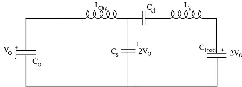
Equivalent Circuit where:  $C_o \gg C_{Load} \gg C_s, C_d$
