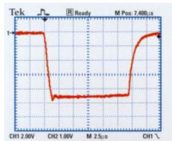
HVPM 100-150 Pulse, 80kV, 90A Into Water Resistor
