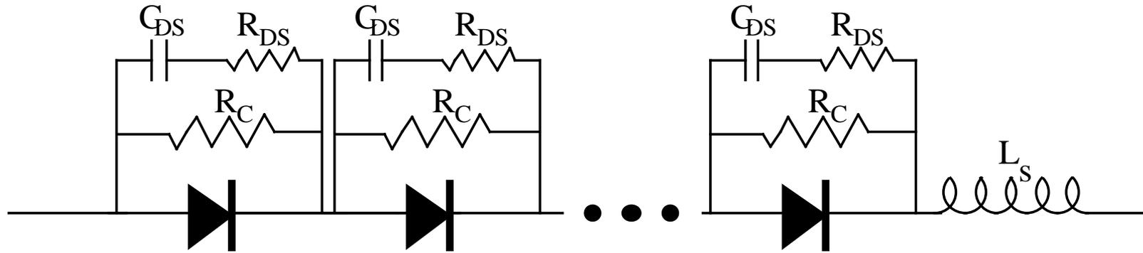
$R_c$  is used for DC grading of diodes to force voltage sharing between diodes. Want the current through  $R_c$  to be large compared to the maximum leakage current ( $I_r$ ) through the diodes:  $R_c \approx \frac{V_{Diode}}{10I_r}$
