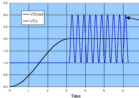
Peak inverse diode voltage  $\sim 2V_o$  instead of  $V_o$
