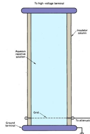
Figure 9.54 Balanced voltage divider with water solution resistor.
