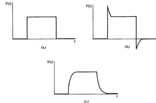
**Figure 9.52** Waveforms from resistive voltage divider. (a) Ideal output voltage from a square-pulse input. (b) Output with significant shunt capacitance. (c) Output with significant series inductance.
