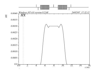
The curly-H function is much smaller in the DBA lattice than in the FODO lattice.
