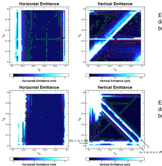
Emittance growth in the TESLA damping ring lattice without coupling bumps (from tracking in SAD).
