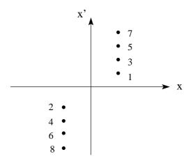
A storage ring is brazenly attempting to operate at a half-integer tune. Alas, there is a gradient error in the machine. A particle is tracked for eight turns, and its phase space evolution at the location of the gradient error is shown in the figure above. The numbers indicate which successive turn corresponds to each point. Explain the phase space plot.
