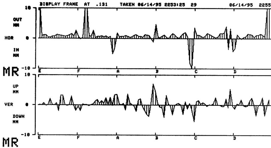
Figure 3: Horizontal and vertical closed orbits in the (now extinct) Main Ring at Fermilab.
