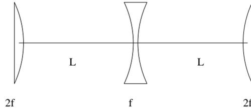
Figure 4: FODO cell, starting and ending in the center of the focusing quadrupole.
