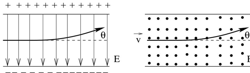
Figure 1: The left figure shows a negatively charged particle getting bent in an electrostatic field. The right figure shows a negatively charged particle getting bent in a magnetic field. The magnetic field points out of the page.
