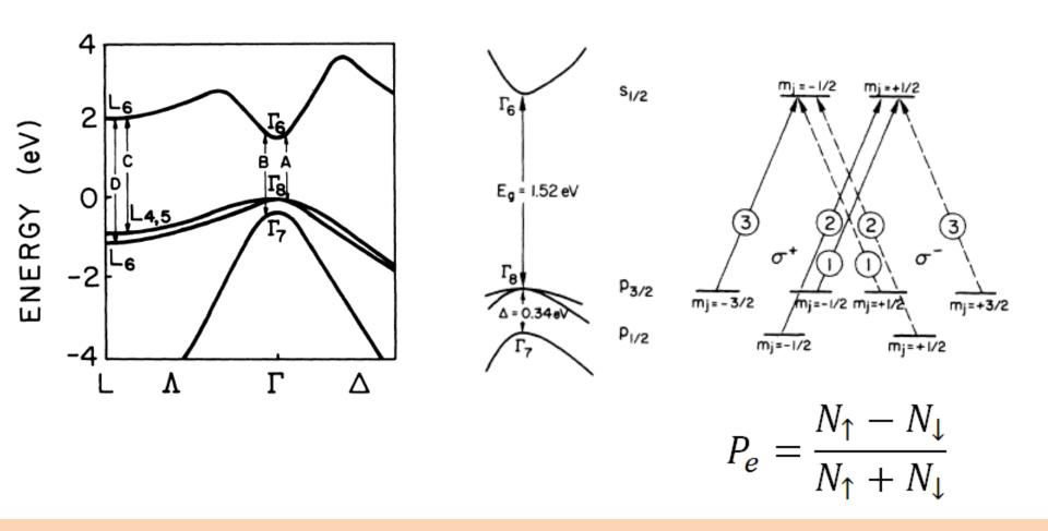
Use light to selectively populate the conduction band with electrons of a particular spin state
