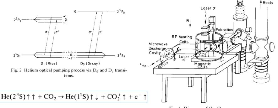
Fig. 1. Diagram of the Orsay source.
