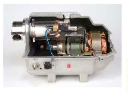
Higher Voltage.... More penetrating x-ray beam Higher e-beam current..... Higher x-ray flux
