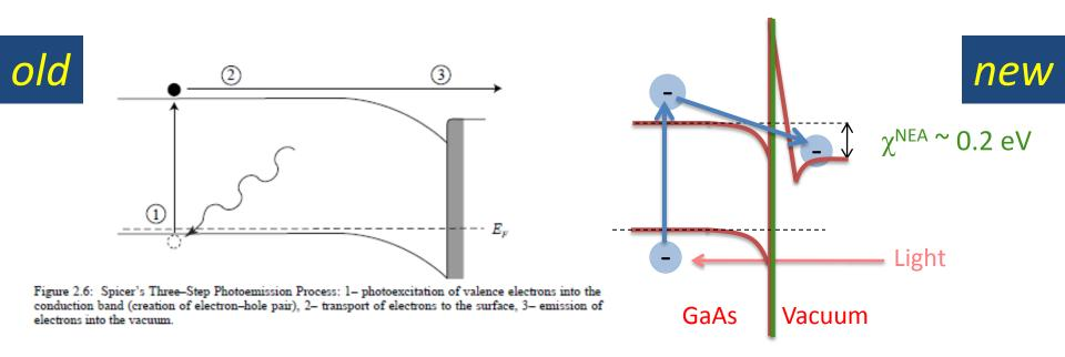
Step 1: Electrons are excited to conduction band by absorbing light
