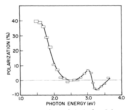
FIG. 6. Spectrum of spin polarization from GaAs + CsOCs at  $T \le 10$  K [the same sample and conditions as curve (a) of Fig. 5]. Note the high value of P=40% at threshold  $(\hbar\omega \sim 1.5 \text{ eV})$  and positive and negative peaks at  $\hbar\omega = 3.0$  and 3.2 eV.
