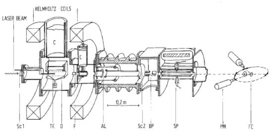
Fig. 3. Longitudinal section of electron source and polarization analyzer. O oven system, F Faraday cup, AL accelerating lens, SP spin precessor (Wien filter), FC foil carrier (details are not shown), PM photo-multipliers, TE test electron source, BP beam steering plates,  $Sc_1$  and  $Sc_2$  positions of scintillators for laser beam adjustment, C cold traps
