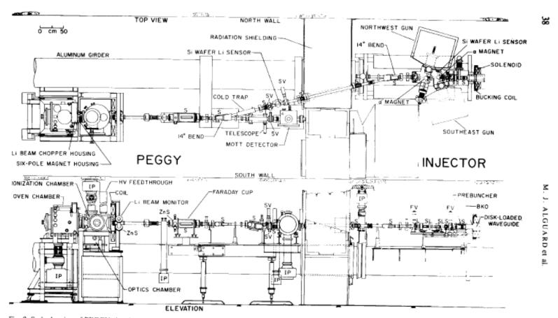
Fig. 9. Scale drawing of PEGGY showing a top view and an elevation. The parallel offset of the PEGGY beam line from the injector beam line can be seen in the top view. Abbreviations which have been used are as follows: BKO, beam knock out for changing pulse duration and separation; FV, fast valve; IP, ion pump; L, magnetic lens; S, magnetic steering; SV, slow valve; T, toroid beam current monitor; and ZnS, zinc sulfide screen for visual monitoring of the beam.
