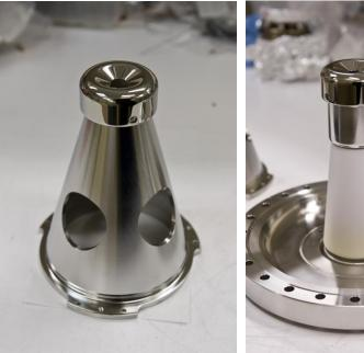
Conventional geometry: cathode electrode mounted on metal support structure
