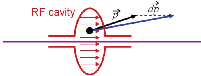
Fortunately, RF cavities are usually designed to provide a longitudinal electric field, so that particles experience a change in longitudinal momentum as they pass through, without any change in transverse momentum.
