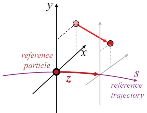
$z$  is *approximately* the distance along the reference trajectory that a particle is ahead of a reference particle travelling along the reference trajectory with momentum  $P_0$ .
