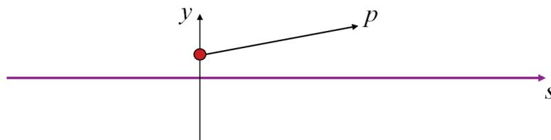
The radiation emitted by a relativistic particle has an opening angle of  $1/\gamma$ , where  $\gamma$  is the relativistic factor for the particle.
