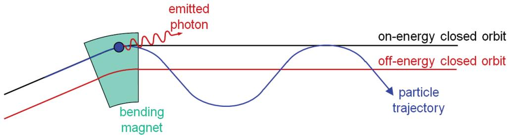
The beam eventually reaches an equilibrium distribution determined by a balance between the radiation damping and the quantum excitation.
