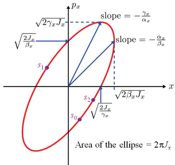
Applying simple geometry to the phase space ellipse, we find that the action (for uncoupled motion) is related to the Cartesian variables for the particle by:
