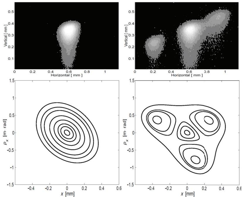
Effect of third-integer resonance on beam distribution. Top: SR light monitor images. Bottom: (simulated) horizontal phase space.
