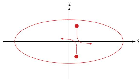
If the energy deviation of either particle following the collision is outside the energy acceptance of the storage ring, then the particle will be lost from the beam.
