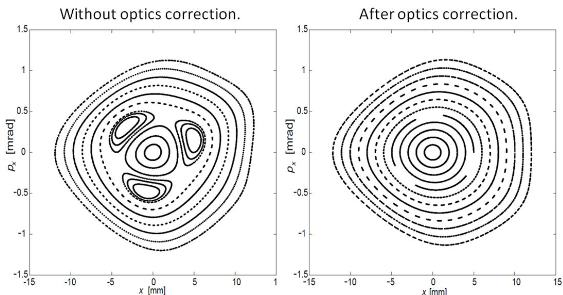
Horizontal phase space in the ALS, close to a third-integer resonance, produced by tracking in a model of the lattice.
