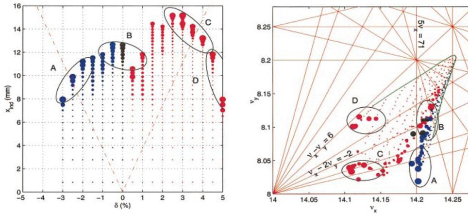
Left: Particle loss as a function of energy deviation (horizontal axis) and horizontal kick amplitude (vertical axis). Right: corresponding points in tune space.
