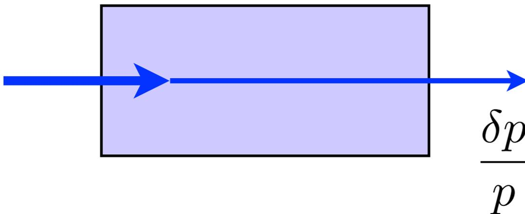
*Some protons escape from the collimator with a reduced “rigidity” after losing energy through inelastic interactions.*
