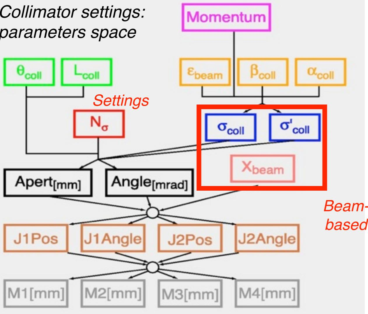
$$\text{jaw} = x_{\text{beam}} \pm n_0 \times \sigma_x$$
