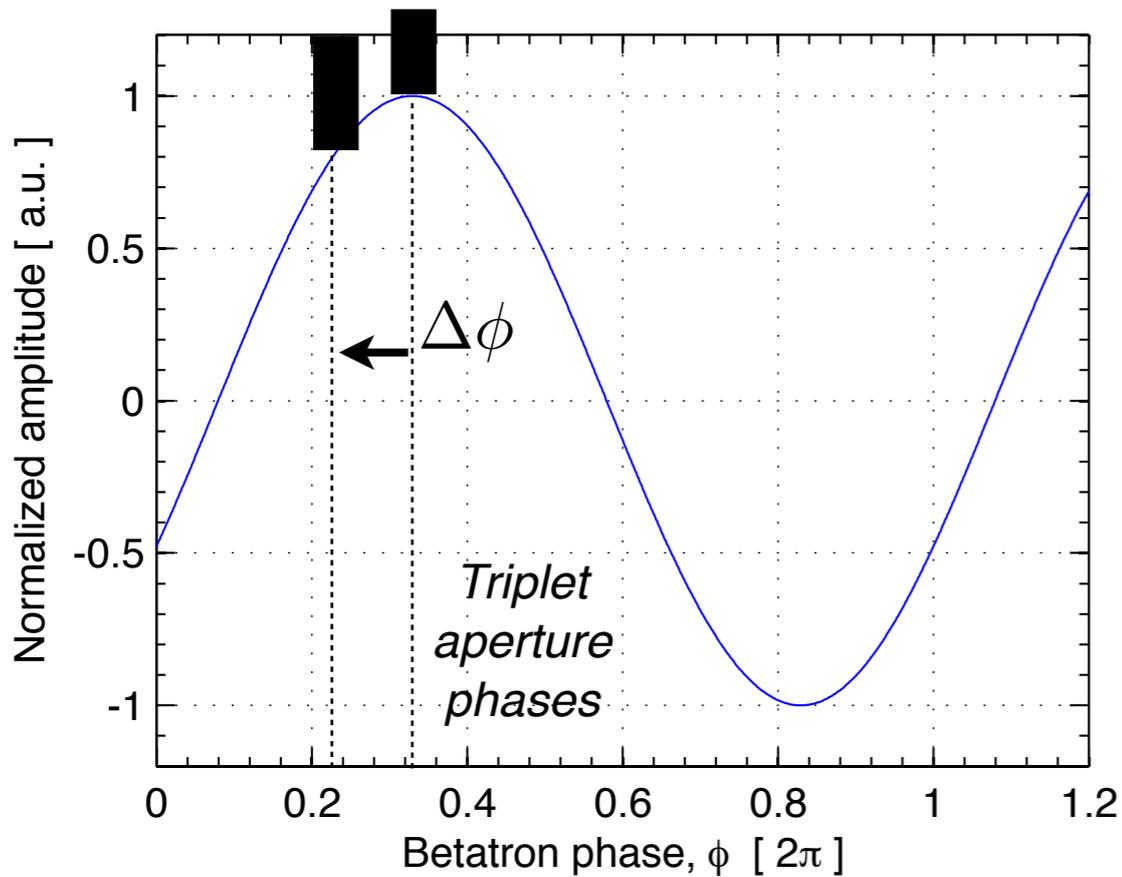
*If one cannot install the TCT at the same phase at the aperture bottleneck, equivalent protection levels can only be achieved **closing the collimator to smaller gaps.***
