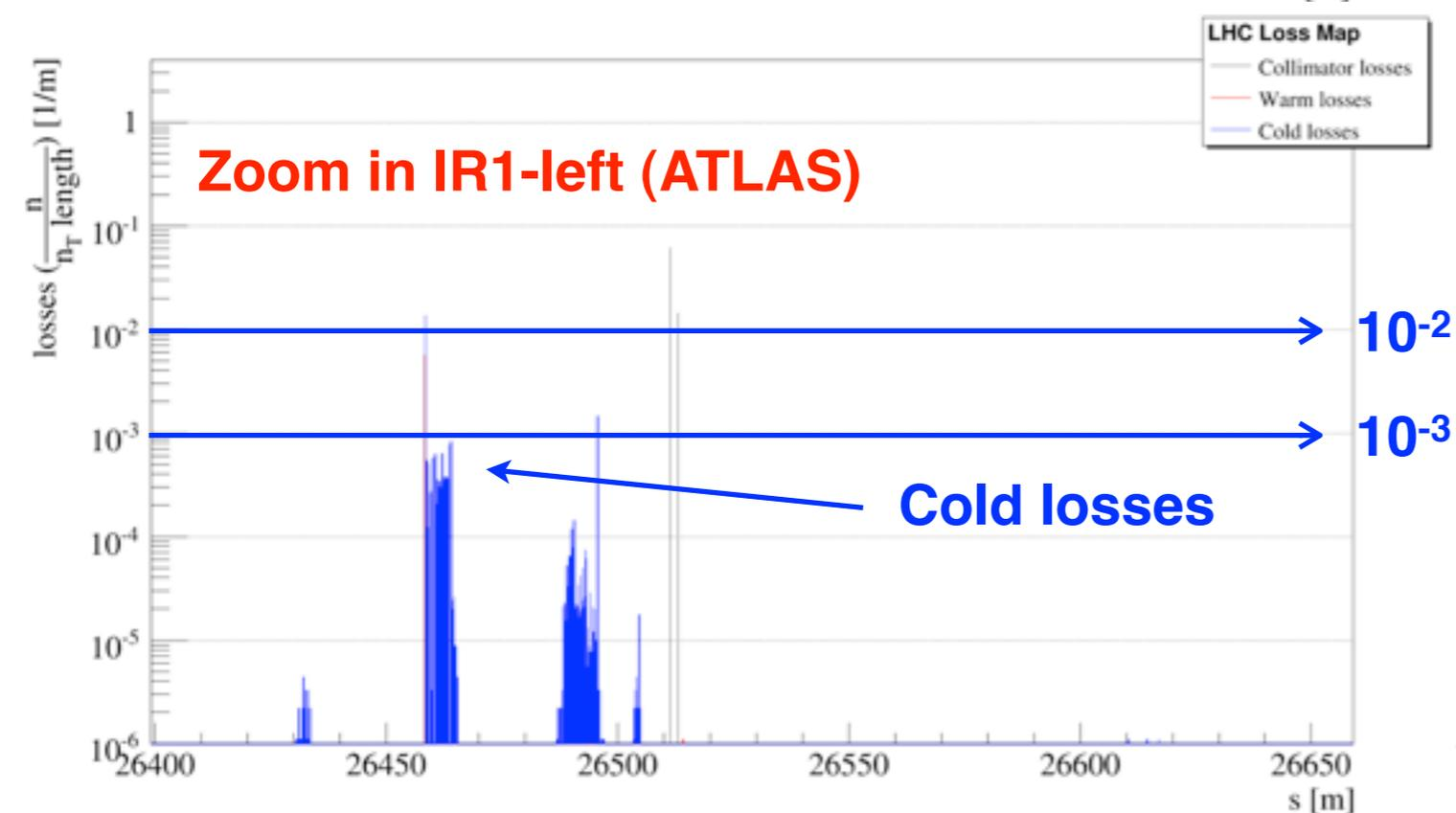
**Single-stage cleaning is apparently not adequate for the LHC needs!**
