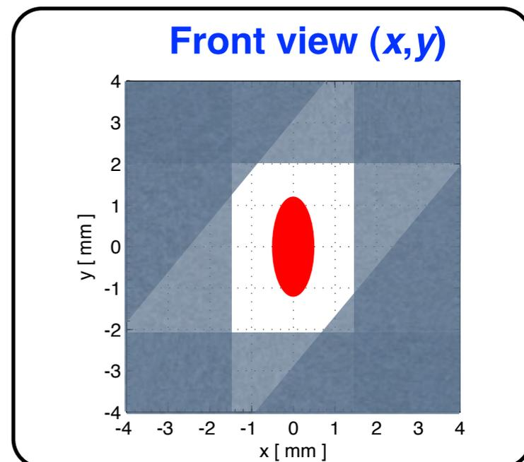
Collimator settings and aperture are expressed in normalized units, using the of local betatron beam size → enable to define the setting “hierarchy”!
