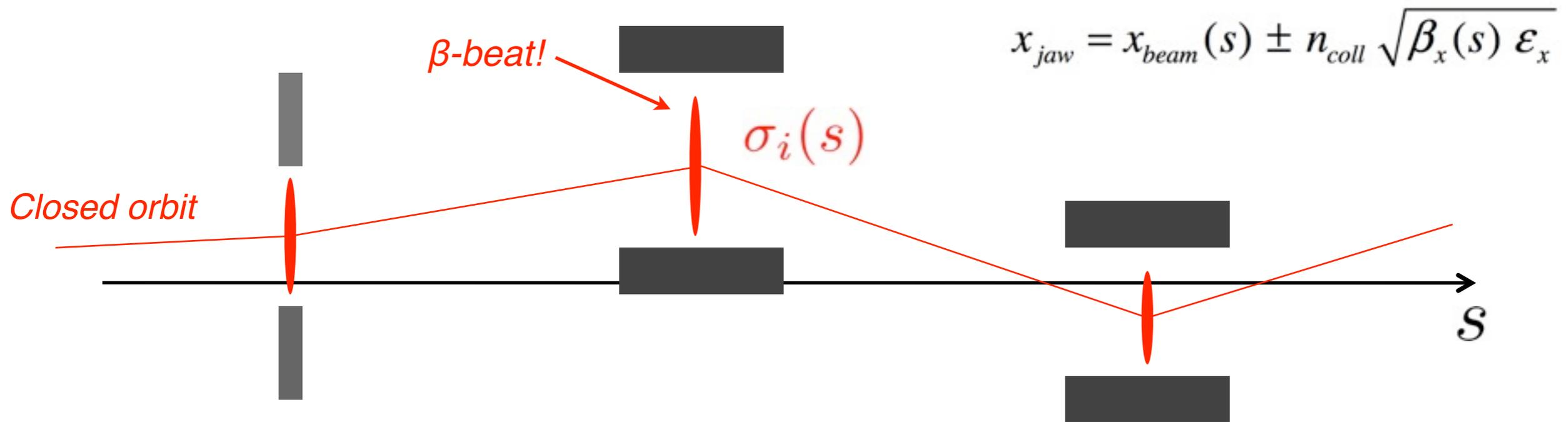
Due to the **very small gaps** involved, collimators cannot be set deterministically using nominal parameters: alignment errors, orbit imperfections and optics errors cause uncertainties large compared to gaps.
