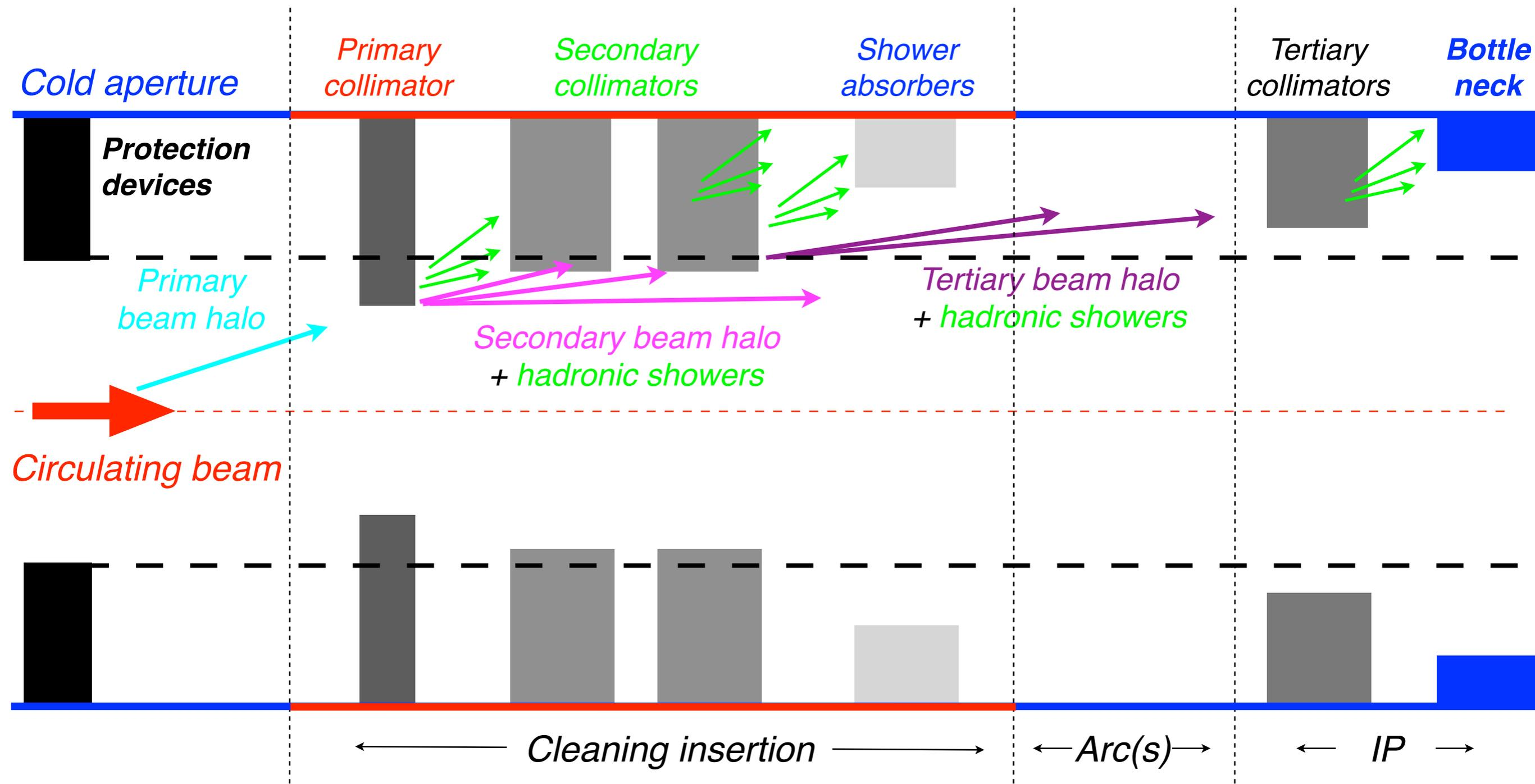
Including protection devices, a **5-stage cleaning** is required!
