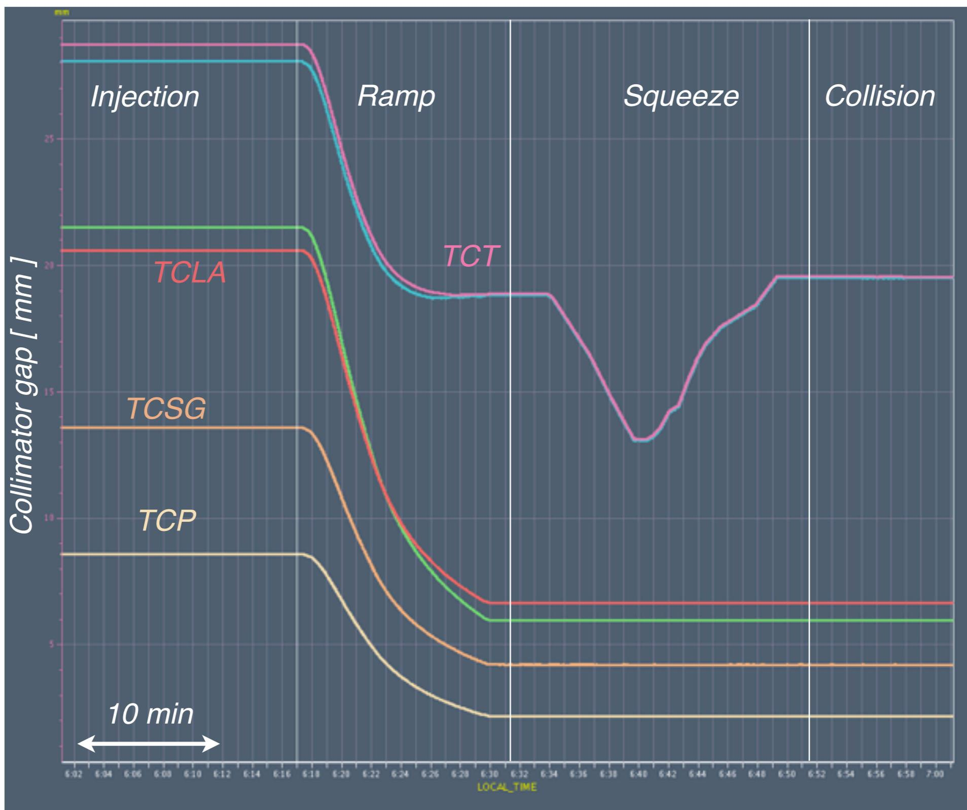
At the LHC, collimator are moved through setting functions versus time.
