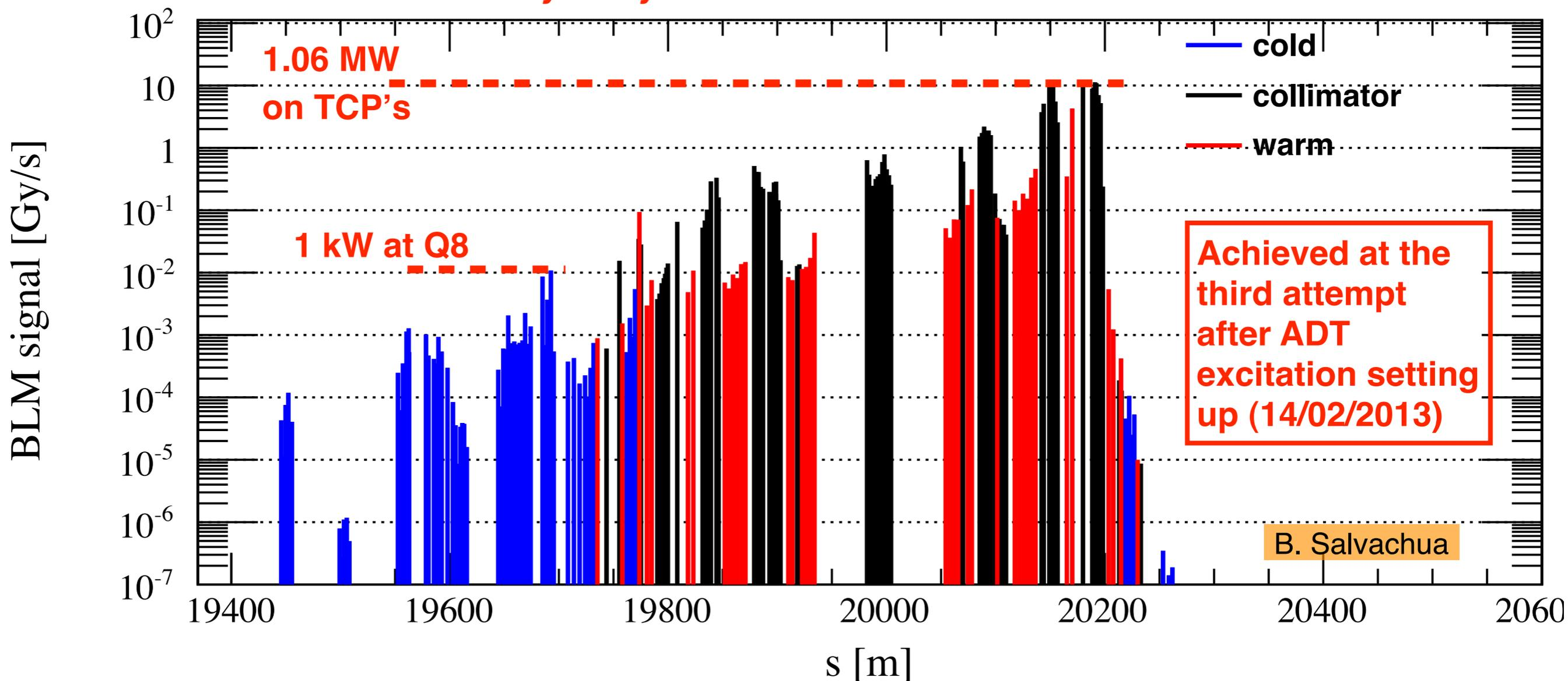
Controlled beam excitation over several seconds: **Peak > 1MW on TCP!**
