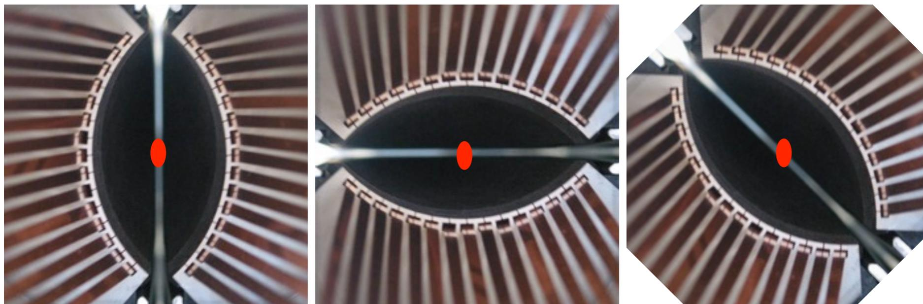
**3 primary collimators** are needed to protect the machine against transverse betatron losses.
