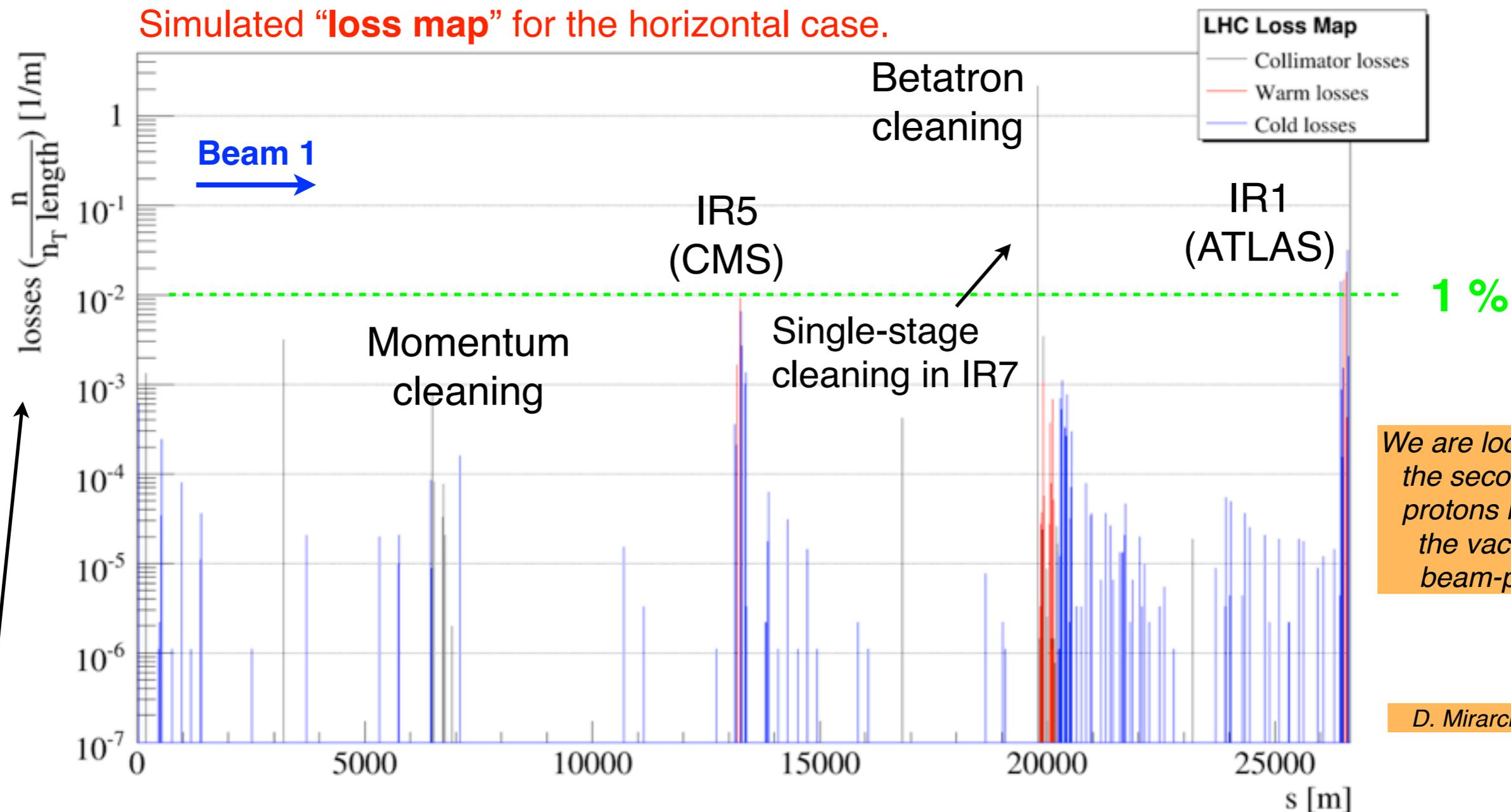
We are looking at the secondary protons lost in the vacuum beam-pipe.
