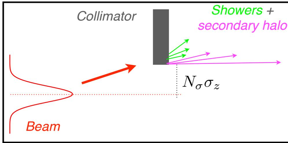
If the “primary” collimator were a black absorber, it would be sufficient to shield the aperture by choosing a gap  $N_\sigma \sigma_z$  smaller than the aperture bottleneck !
