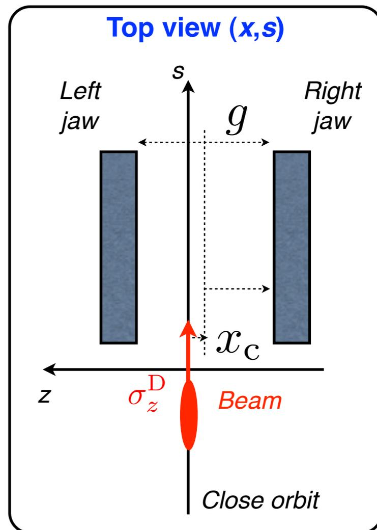
$$\sigma_z^D = \sqrt{\beta_z \frac{\epsilon_z}{\gamma} + D_z \left(\frac{\delta p}{p}\right)^2} : \text{RMS beam size}$$
