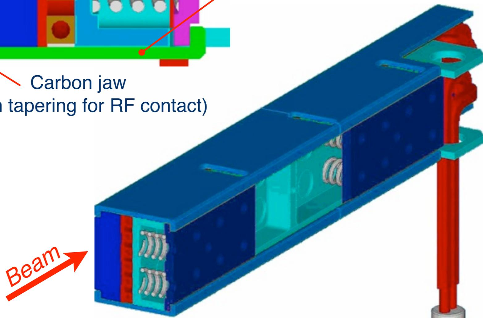
*Special "sandwich" design to minimize the thermal deformations:*
