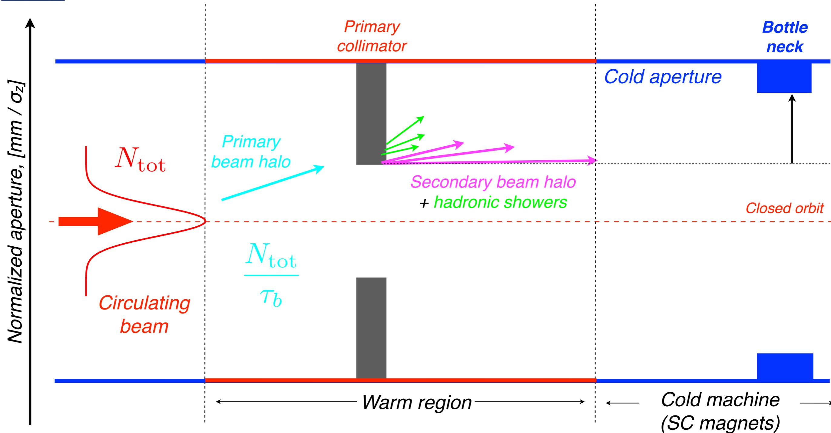
The particles lost from the beam core drift transversally and populate beam tails. Ultimately, they reach the machine **aperture bottleneck**.
