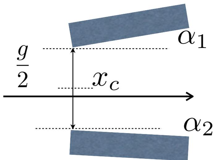
Can apply random errors to collimator geometry.
