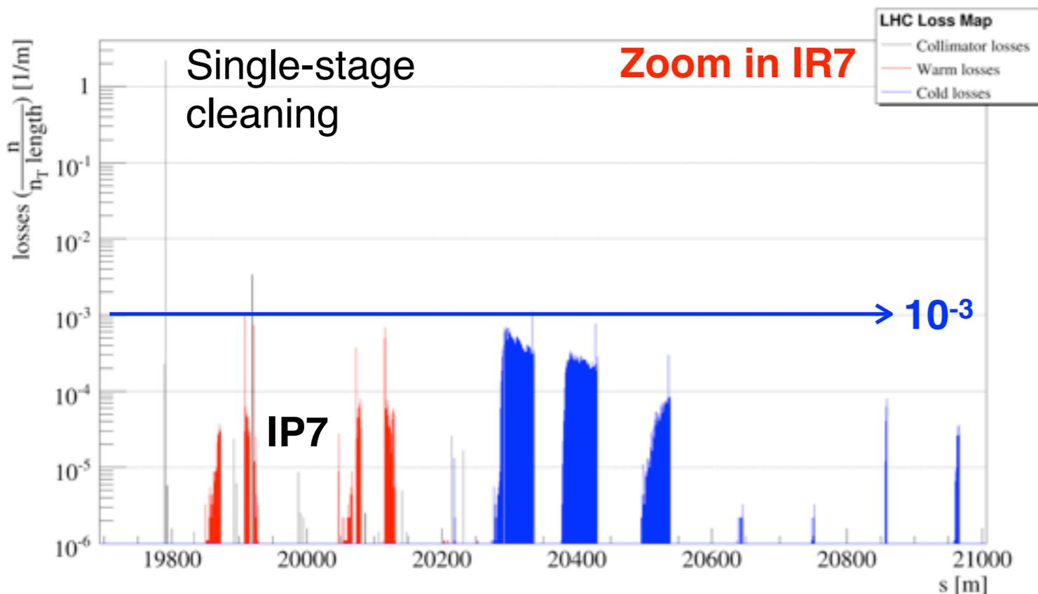
Typical assumed **quench limit** at 7 TeV for steady losses of  $\sim$ second timescales:
