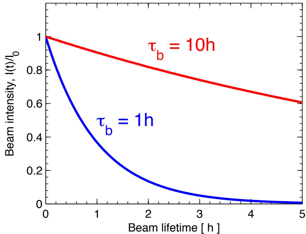
Beam losses mechanisms are characterized by a time-dependent **beam lifetime** during the machine cycle. This measures the **total beam losses** that a collimation system must handle.
