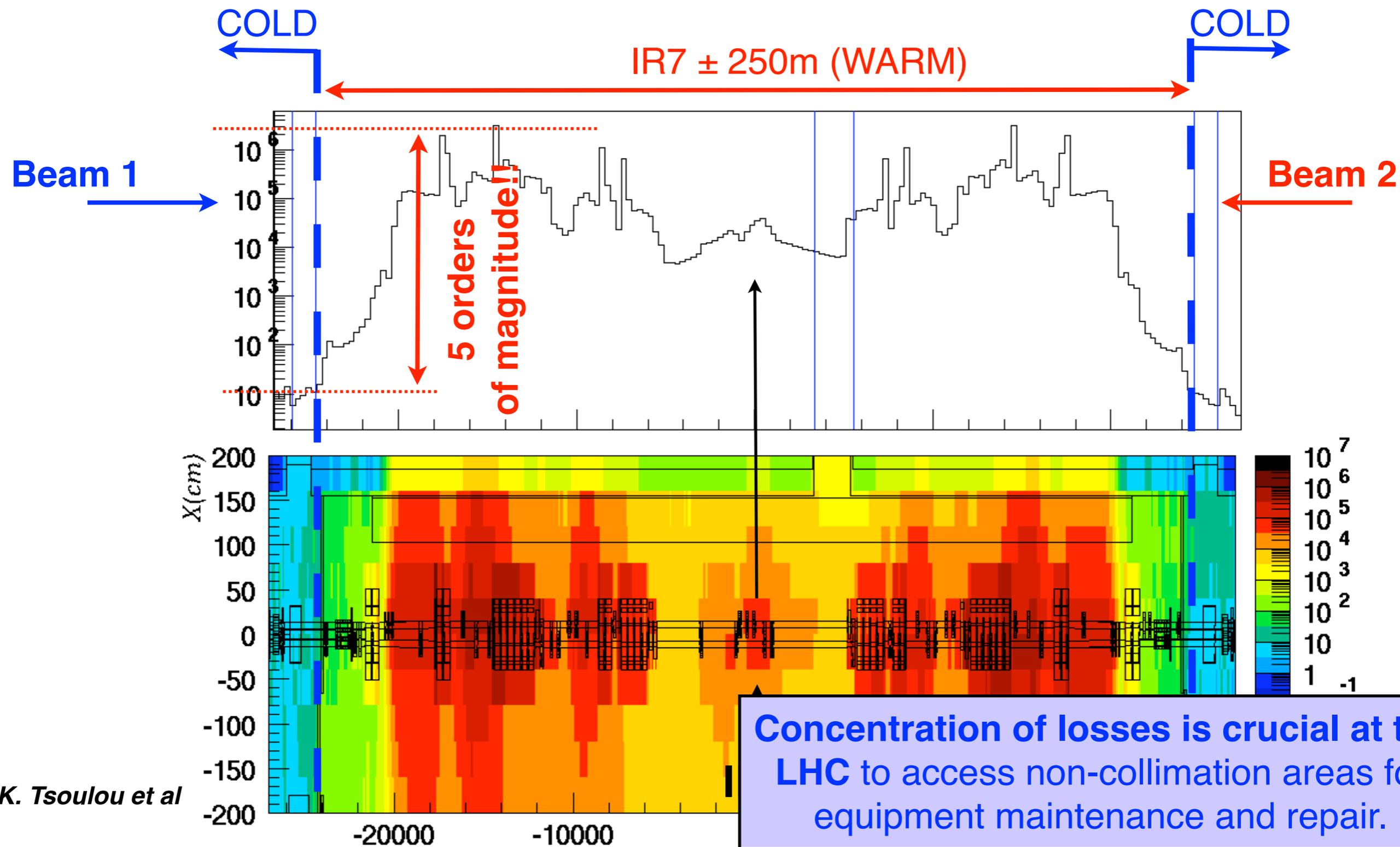
**Activation from halo losses is basically confined within the warm insertions!**
