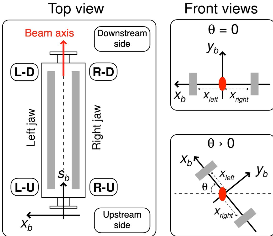
In the LHC, we also have “rotated” collimators that provide collimation in the **skew plane**.
