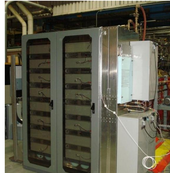
Dust causing frequent failures on TEVATRON QP electronics )copied from H. Edwards/P. Czarapata, FNAL, Groemitz Miniworkshop 2005
