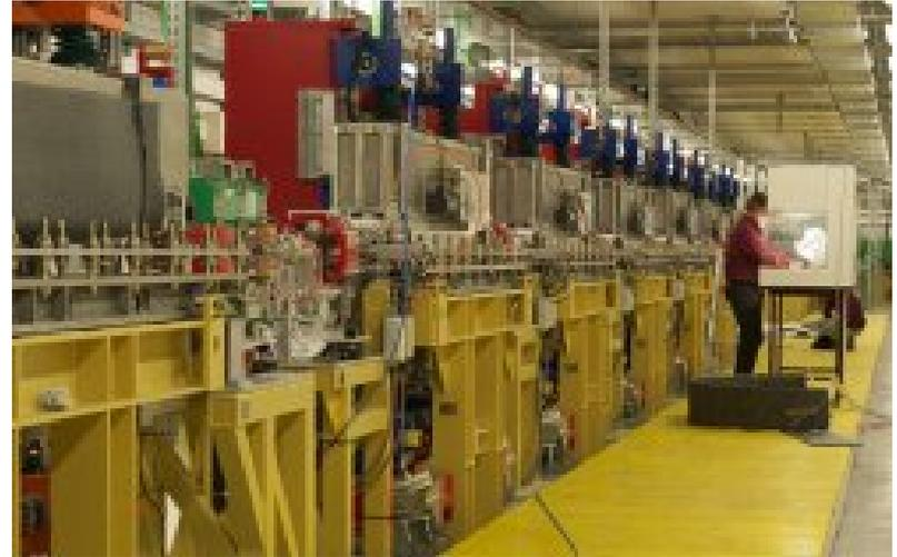
Fermi@Elettra is an FEL user facility in Trieste, Italy that uses the HGHG mechanism to produce coherent FEL pulses at wavelengths down to 43 nm. The electron beam is seeded with a 258 nm laser, and then a single HGHG stage produces radiation at the 6<sup>th</sup> harmonic. A delay line is used so that a “fresh” part of the electron bunch is seeded with the 43 nm radiation (more on this later).
