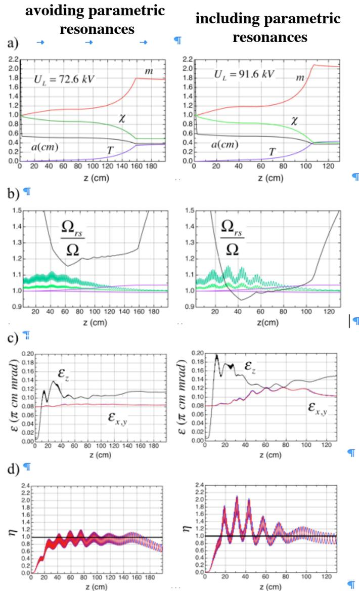
Fig. 4. Beam dynamics in RFQ with beam current  $I = 35$  mA: (left) avoiding parametric resonances, (right) including parametric resonances: (a) RFQ parameters, (b) parametric resonance bandwidth: (green) Eq. (18), (red) Eq. (9), (c) beam emittances, (d) equipartitioning parameter, Eq. (5).
