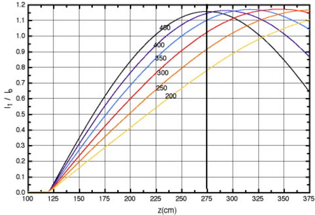
The first harmonic of the induced beam current in the second gap as a function of  $z$  for different values of voltage at first gap  $\frac{I_1}{I} = 2J_1(X)$
