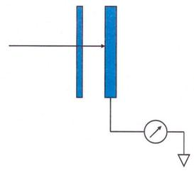
Schematic of the phase scan measurement setup
