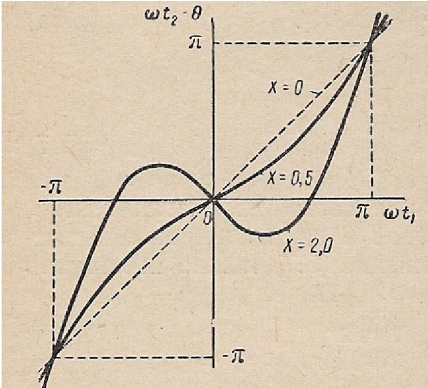
Phase of arrival of particle into second gap as a function phase of the same particle in the first gap.
