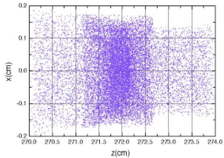
Effect of space charge repulsion on beam bunching.
