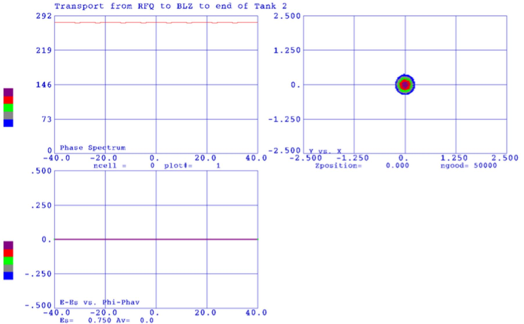
Example of beam dynamics in accelerating structure. (Courtesy of Larry Rybarcyk.)
