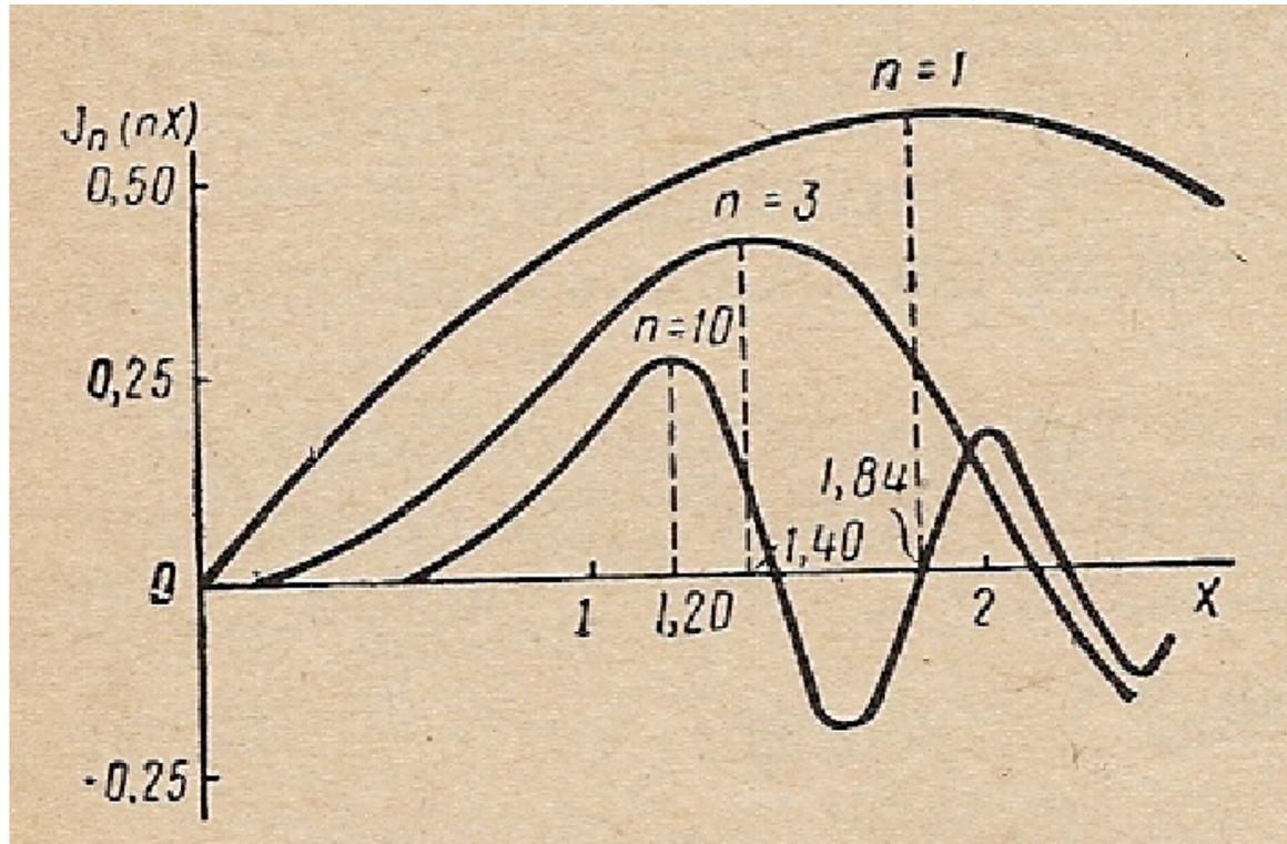
Bessel functions determine amplitude of the first, third and tenth harmonics of induced current in two-resonator buncher.
