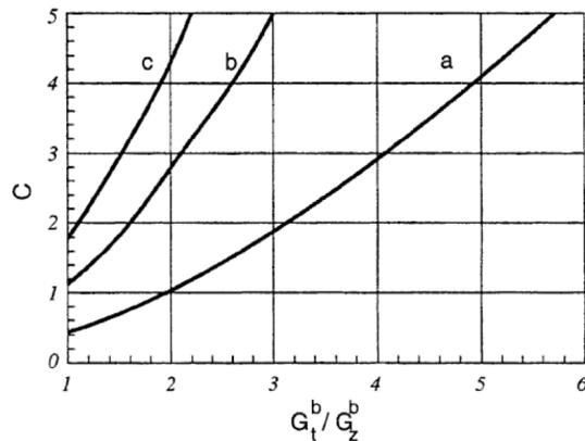
Coefficient  $C$  in bunch shape for  $\varphi_s = -30^\circ$  as a function of ratio of transverse and longitudinal gradients of space charge field of the beam: a)  $\gamma = 1$ , b)  $\gamma = 3$ , c)  $\gamma = 6$ .
