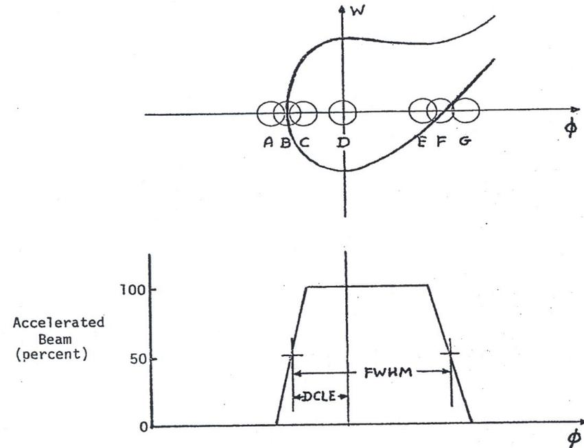
Accelerated beam as a function of beam phase
