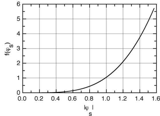
Fig. 5.7. Function  $f(\varphi_s) = 3\varphi_s \sin\varphi_s - \frac{9}{2} \varphi_s^2 \cos\varphi_s + \cos\varphi_s - \cos 2\varphi_s$  in maximum beam current, Eq. (5.118).
