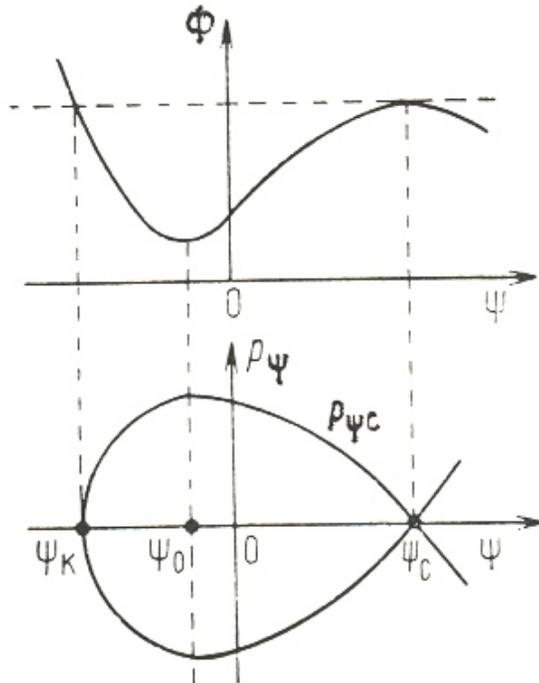
The potential function and separatrix of the beam with high space-charge density (from Kapchinsky, 1985).
