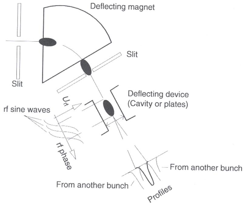
Fig. 7.1. Simplified scheme to measure longitudinal emittance
