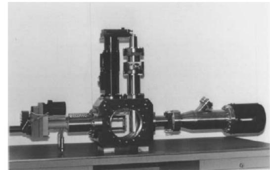
Figure 4: 3D-BSM for CERN Linac-2.
