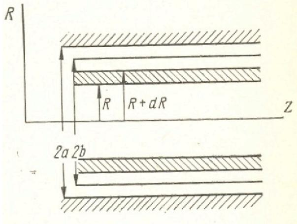
Reduced plasma frequency of the beam of radius  $R$  in the tube of radius  $a$   $\omega_q = \sqrt{F_p} \omega_p$
