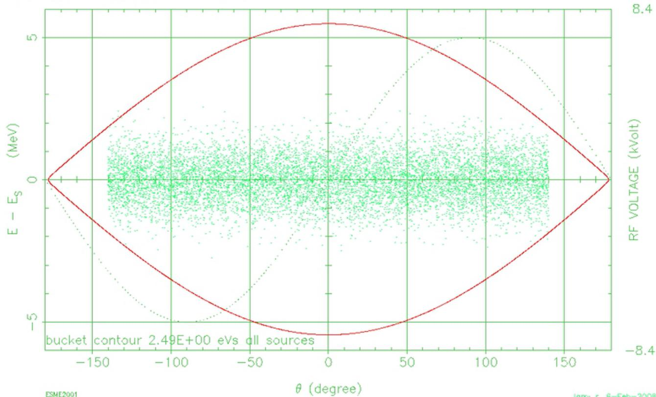
Longitudinal oscillations in RF field with  $\varphi_s = -90^\circ$ . (Courtesy of Larry Rybarczyk.)
