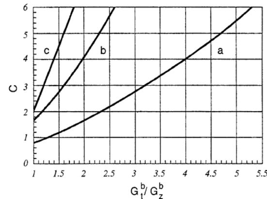
Coefficient  $C$  in bunch shape for  $\varphi_s = -60^\circ$  as a function of ratio of transverse and longitudinal gradients of space charge field of the beam: a)  $\gamma = 1$ , b)  $\gamma = 3$ , c)  $\gamma = 6$ .
