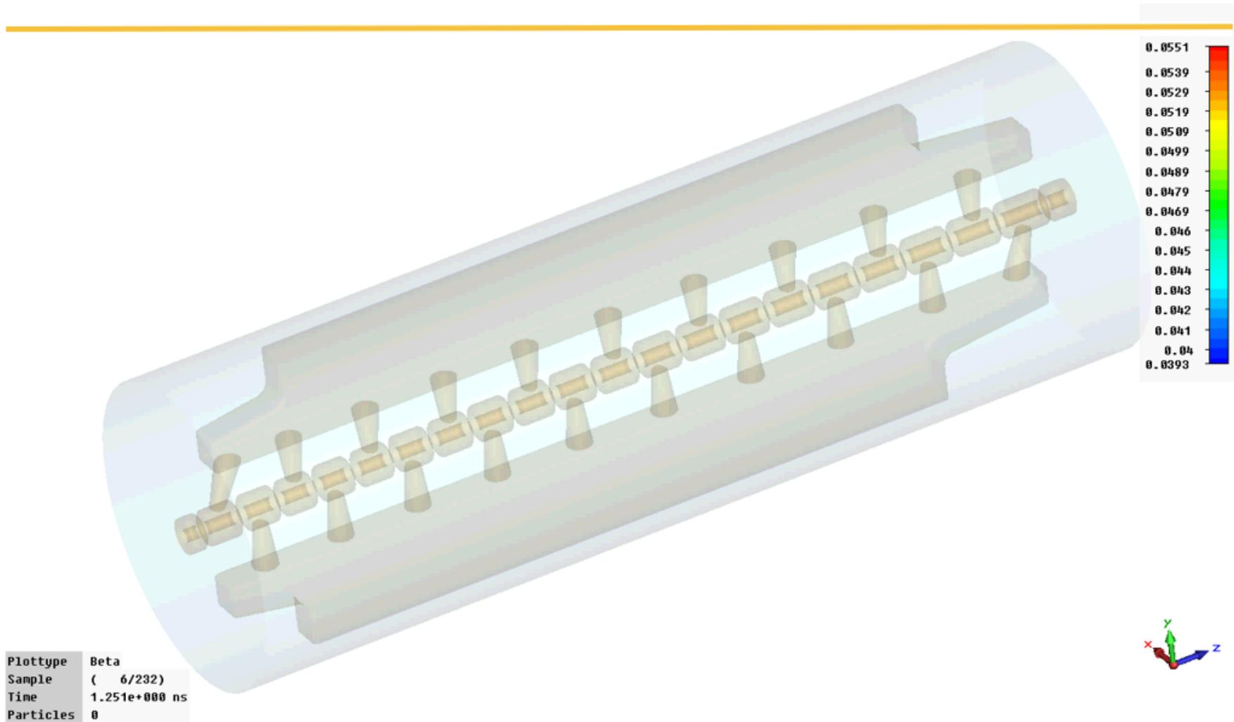
Dynamics of elliptical beam injected into RF linac (courtesy of Sergey Kurennoy).
