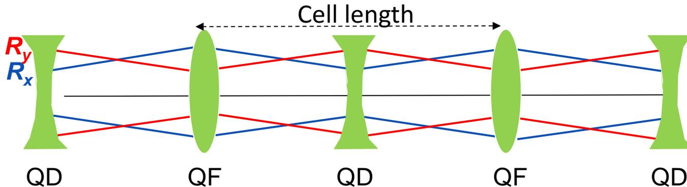
FODO lattice with  $90^\circ$  phase advance (one oscillation = 4 cells)
