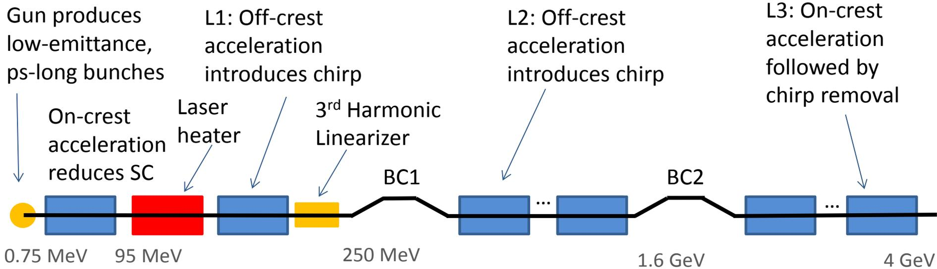
Layout of LCLS-II Linac (mostly superconducting L-band)
