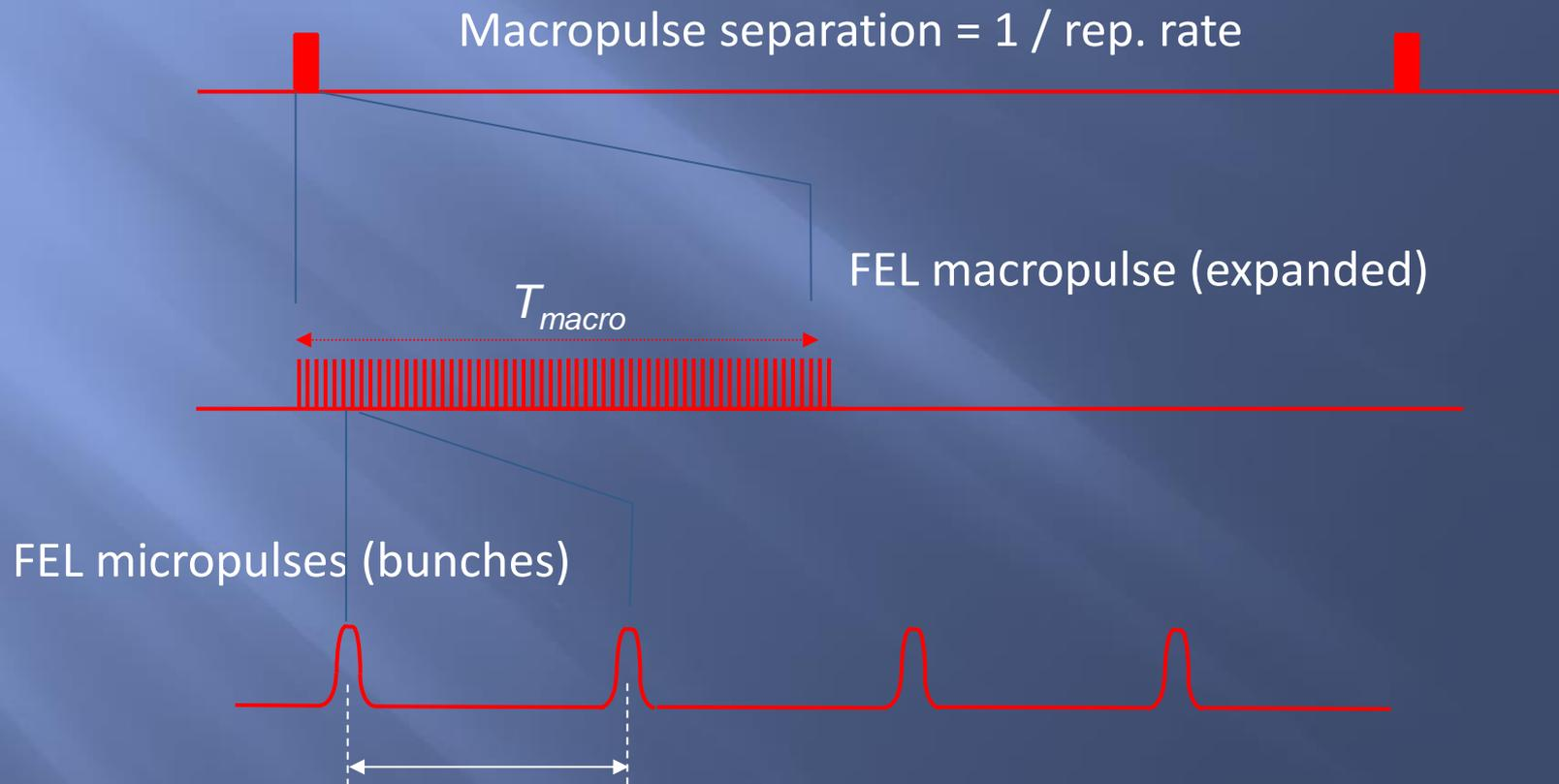
Micropulse separation =  $n (1 / \text{RF})$
