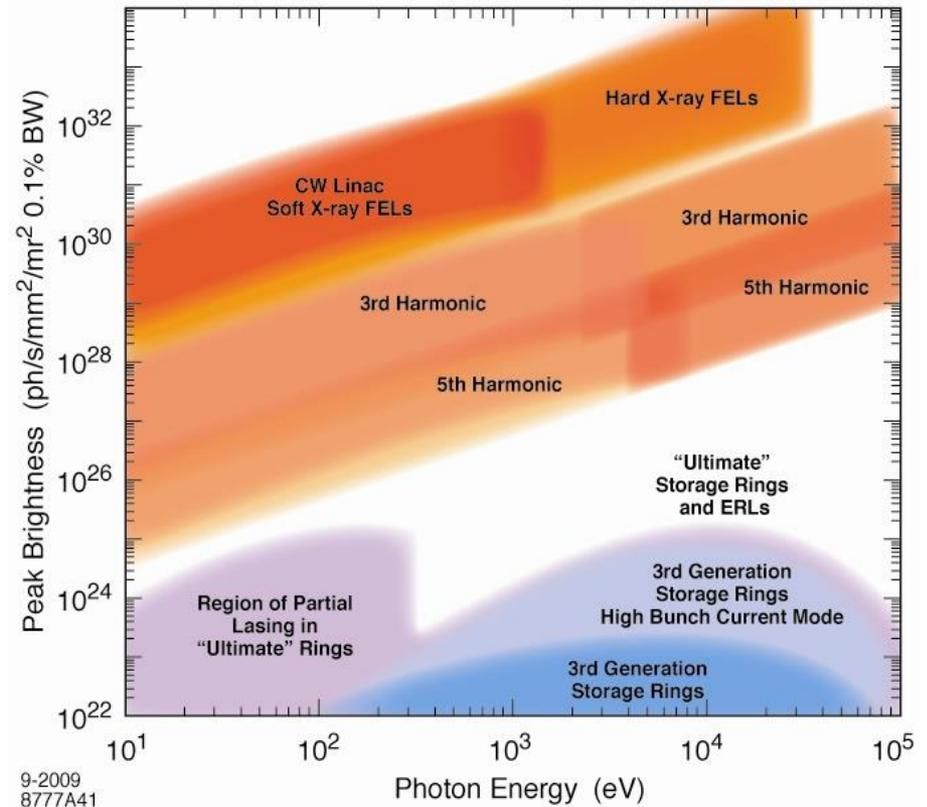
Peak brilliance of linac-based 4<sup>th</sup> generation light sources (XFEL) is ten orders of magnitude above that of the 3<sup>rd</sup> generation light sources and more than 20 orders of magnitude above Bremsstrahlung sources.
