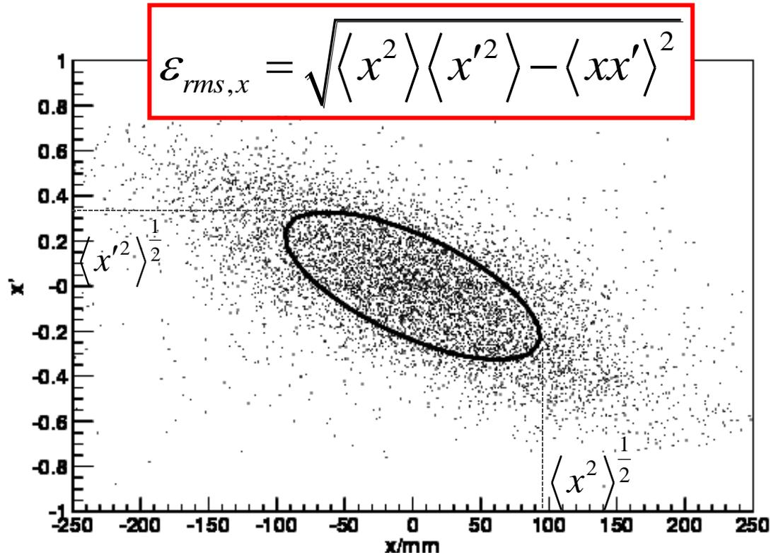
Beams are treated as a statistical distribution of particles in  $x'-x$  (also in  $y'-y$  and  $\gamma-ct$ ) trace space. We can draw an ellipse around the particles such that 50% of the particles are found within the ellipse. The area of the ellipse is  $\pi$  times the rms beam emittance, which is defined in the equation above.
