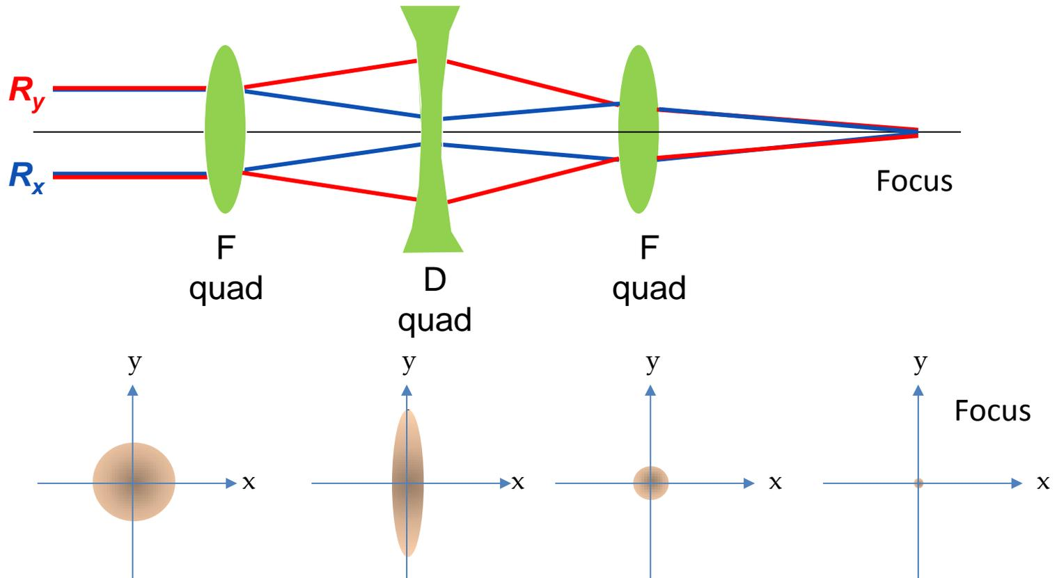
Evolution of electron beam's  $y$ -vs- $x$  profile through a quad triplet
