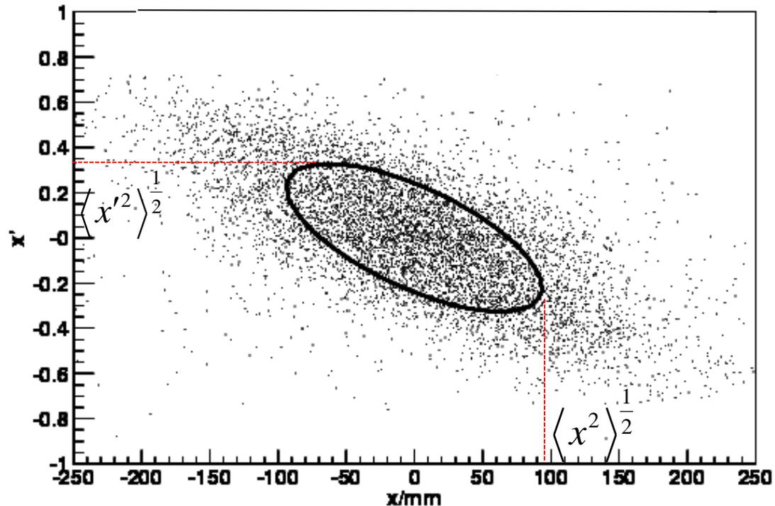
Each particle is represented by a dot in the  $x$ - $x'$  plot where  $x$  and  $x'$  the particle position and angle in  $x$  with respect to the principal trajectory. The above trace space corresponds to a converging beam.
