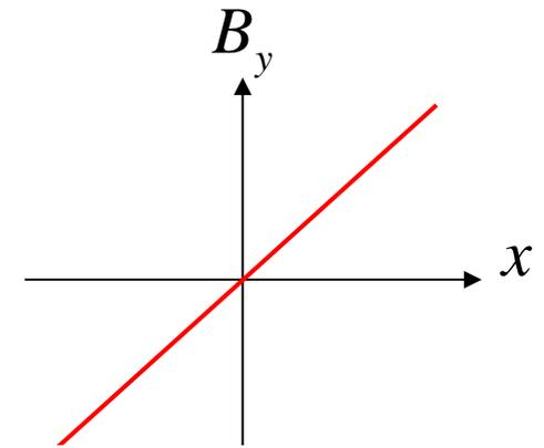
Magnetic field in y increases linearly with x, the deviation from center.
