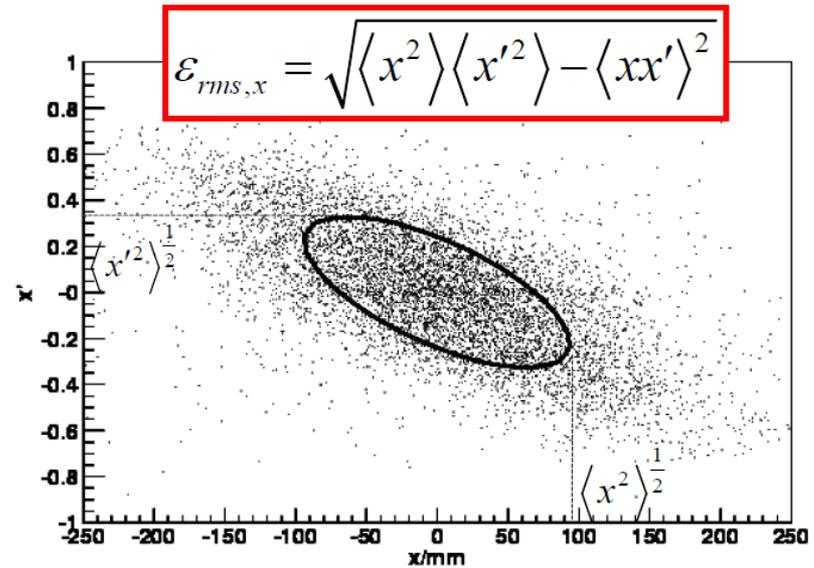
Acceleration reduces  $x'$  by boosting  $p_z$  and reduces the geometric emittance
