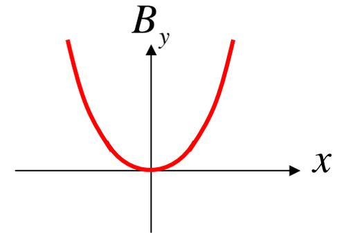
Magnetic field in  $y$  at  $y = 0$  increases with  $x^2$  where  $x$  is the distance from center.
