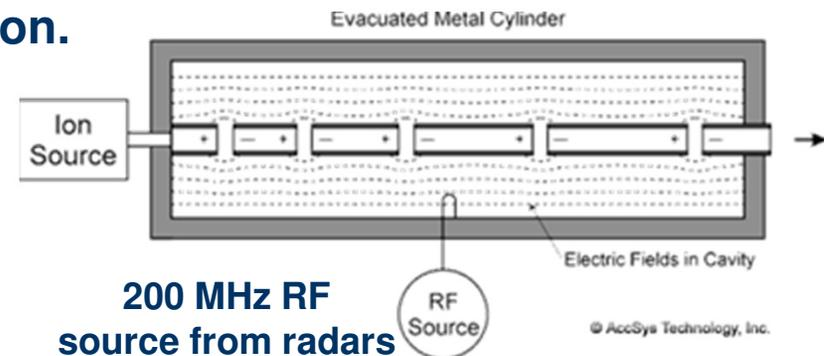
The Alvarez structures are still widely used as pre-accelerator for protons and ions. The particles at few hundred keV from a Cockcroft-Walton for example, are accelerated to few hundred MeV.
