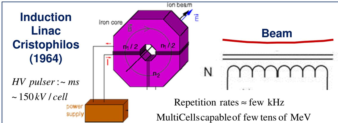
**Induction accelerators can be very efficient (> 50%) and allow for very high currents (~ 1kA) at relatively moderate energies (few tens of MeV)**
