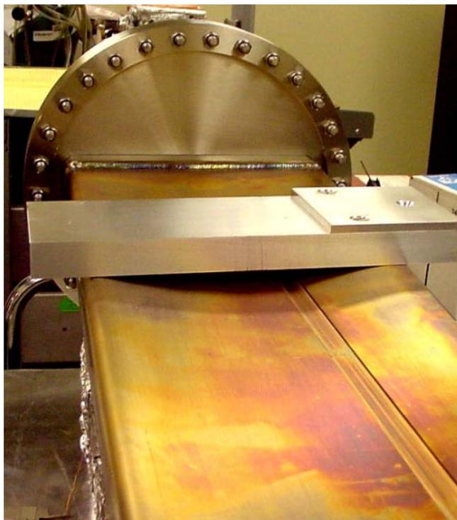
*Distorted copper chamber during a bakeout*
