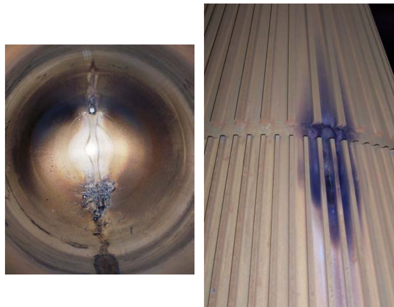
Electron beam melted through aluminum body
