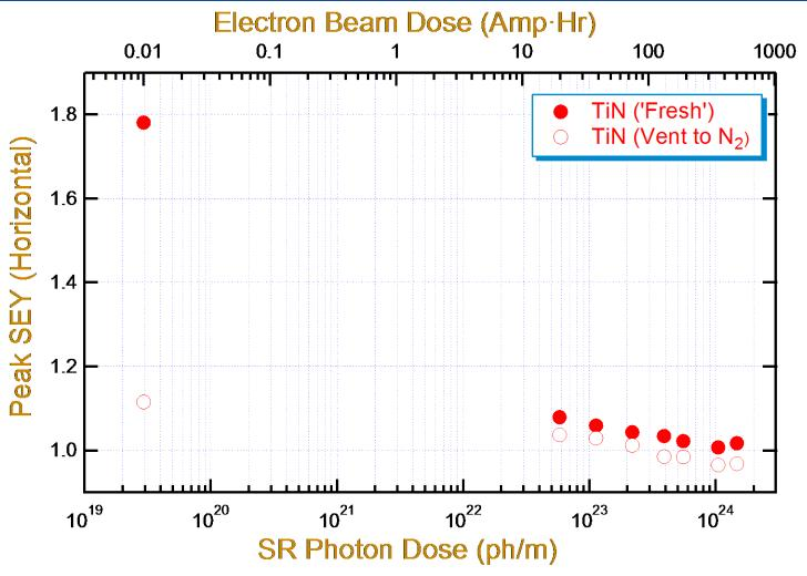
TiN coating has been chosen as the primary SEY-reduction coating for Super KEKB HER, and base design for the ILC e<sup>+</sup> Damping Ring
