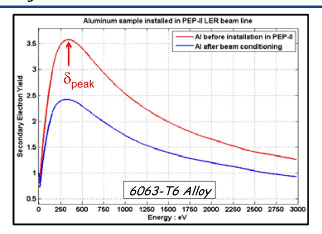
The most commonly used aluminum alloys (6061 and 6063) have very high secondary emission yield (SEY), even with significant 'conditioning'. This is very undesirable for high performance accelerators for positively charged particles, such as ILC  $e^+$  DR, KEK B HER, LHC, etc.
