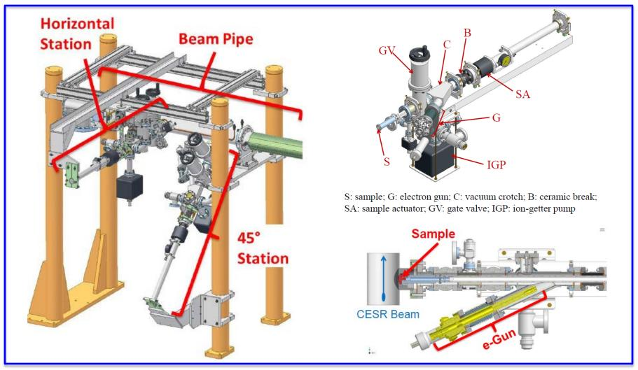
Two SEY stations, with sample load-lock, allow beam (SR) conditioning of samples and in-situ SEY measurement.
