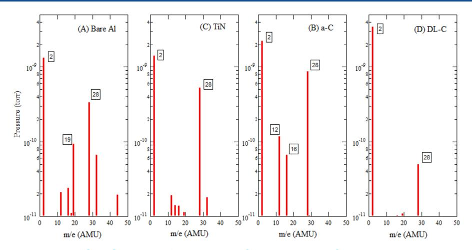
RGA Spectra from Well-Conditioned Chambers with ~400 mA Stored Beam @ 5 GeV
