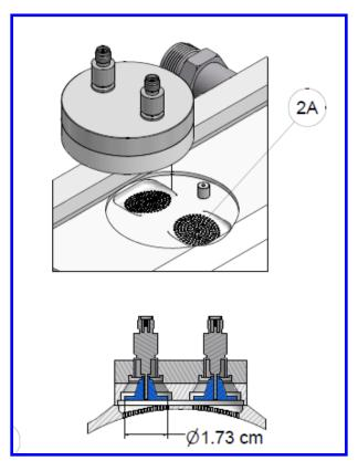
RF-shielded pickups for measuring EC growth
