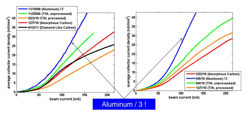
20 bunch train of positrons, 14ns spacing, at 5.3GeV
