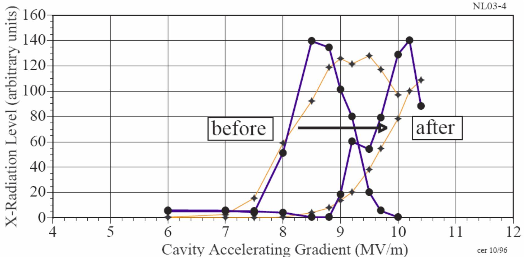
Figure 1. Radiation reduction with He processing.
