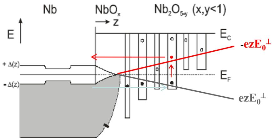
Band structure at Nb-NbO<sub>x</sub>-Nb<sub>2</sub>O<sub>5-y</sub> interfaces
