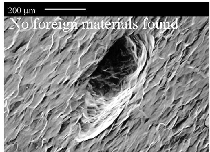
Surface defects, holes can also cause TB
