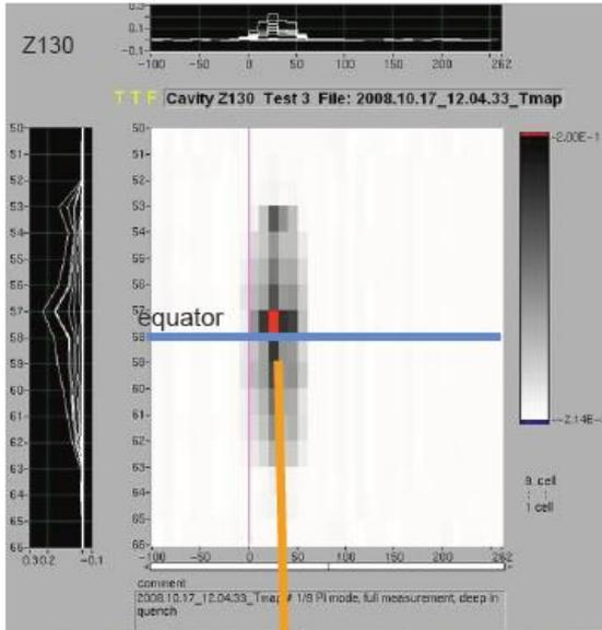
hole in the equator weld
