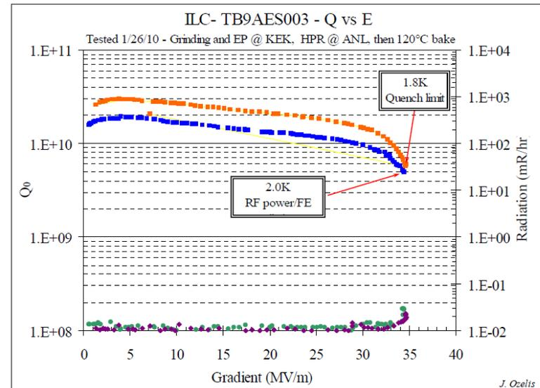
Figure 1.) Q<sub>0</sub> vs E runs at 2.00K and 1.80K.
