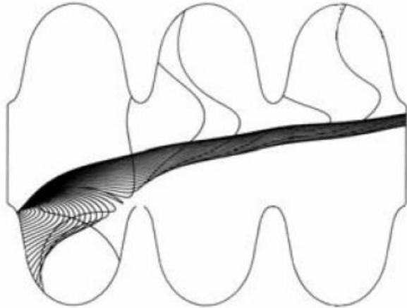
Acceleration of electrons drains cavity energy
