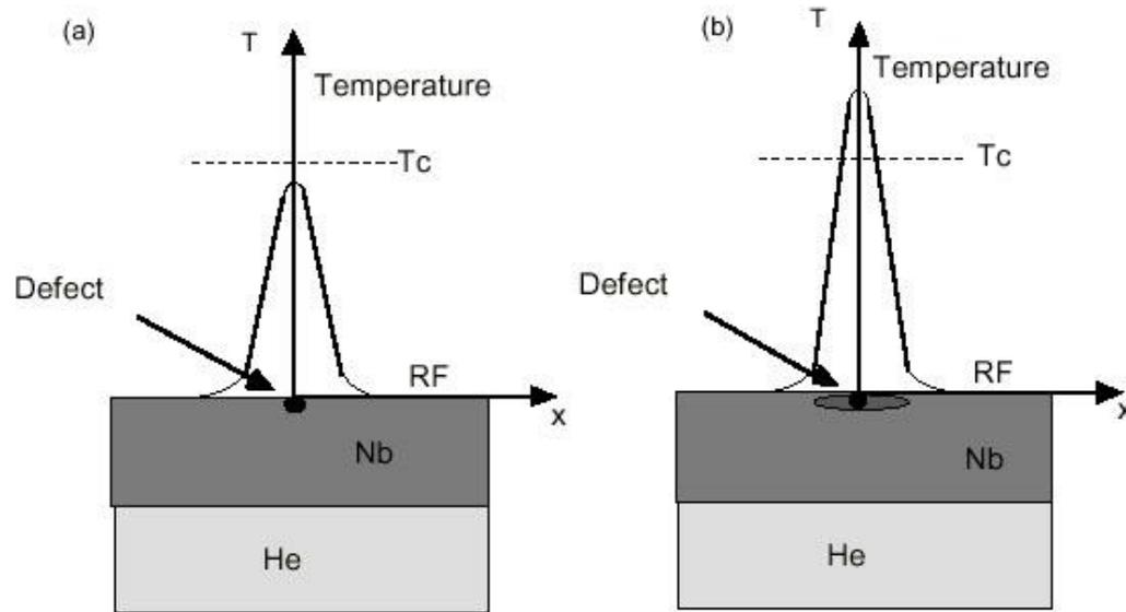
Thermal breakdown occurs when the heat generated at the hot spot is larger than that can be transferred to the helium bath causing  $T > T_c$ : “quench” of the superconducting state
