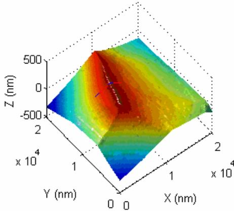
AFM image of a grain boundary edge
