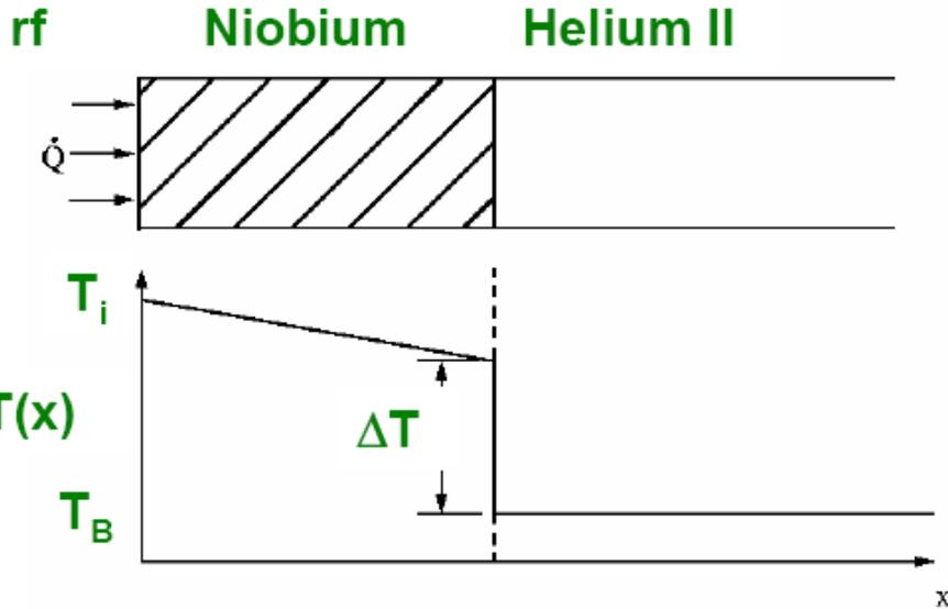
Temperature difference between inner surface and helium bath temperature (two dimensional case):
