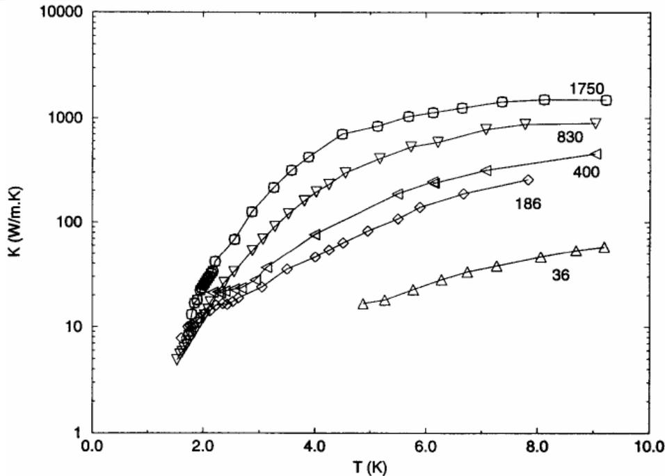
Fig. 3 The thermal conductivity of niobium as a function of temperature, for various RRR values.
