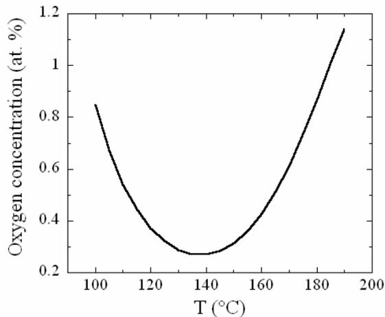
Calculated oxygen concentration at the metal/oxide interface as a function of temperature after 48h baking
