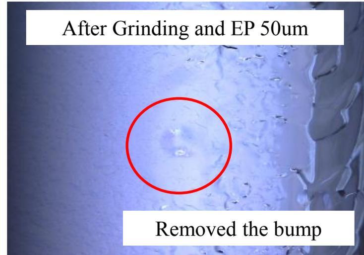
Quench at  $E_{acc} = 20 \text{ MV/m}$
