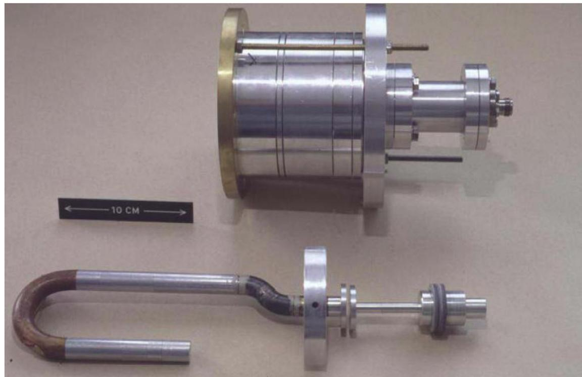
Fig. 1 Geometry of the HOM coupler used in LEP
