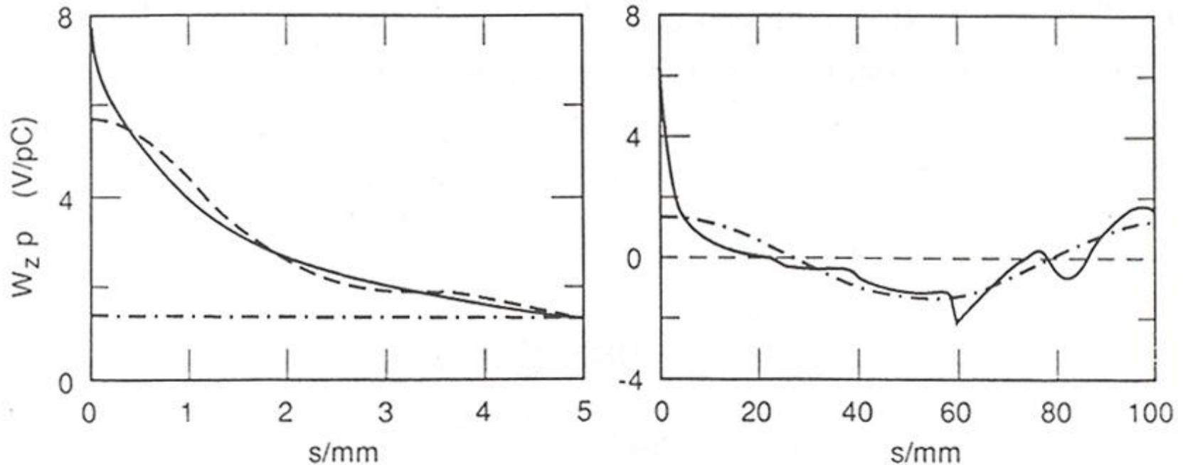
Fig. 10 Longitudinal wake per cell for an average SLAC cell. The solid curve includes an analytical extension for the high frequency behavior.
