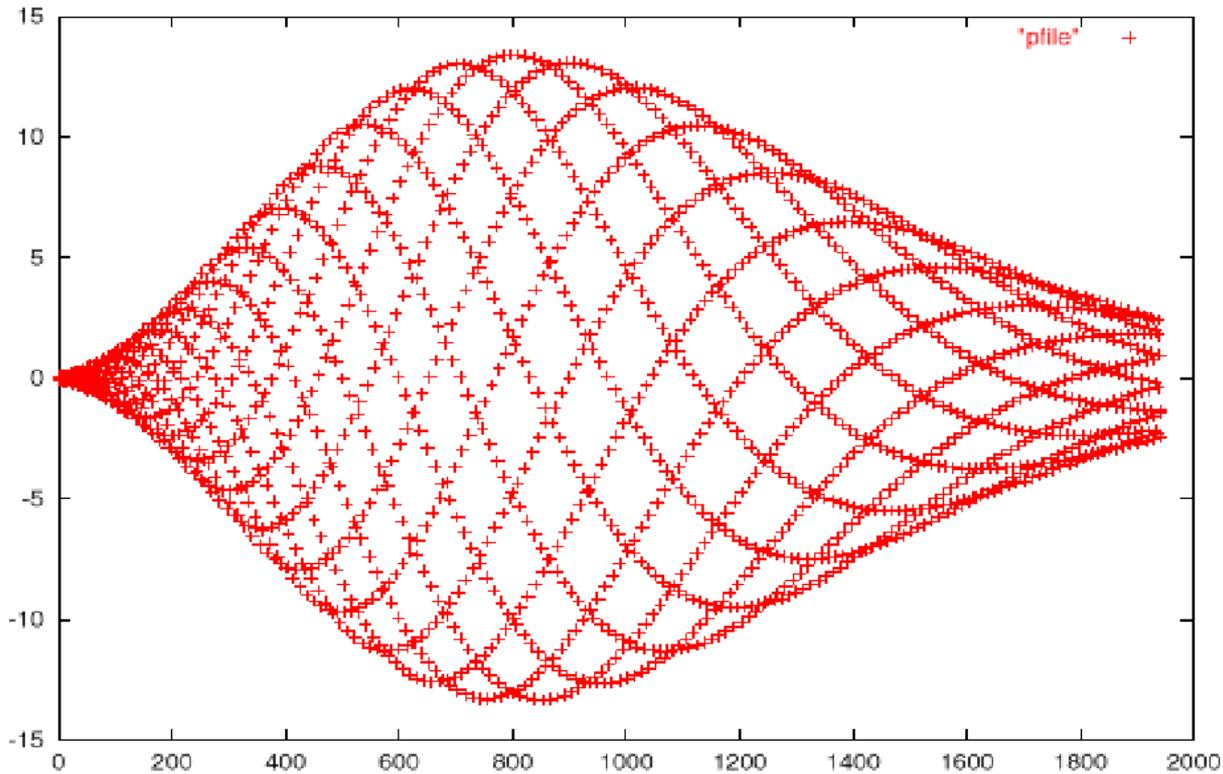
Figure 1: Plot of transverse beam centroid displacement at the end of the linac.
