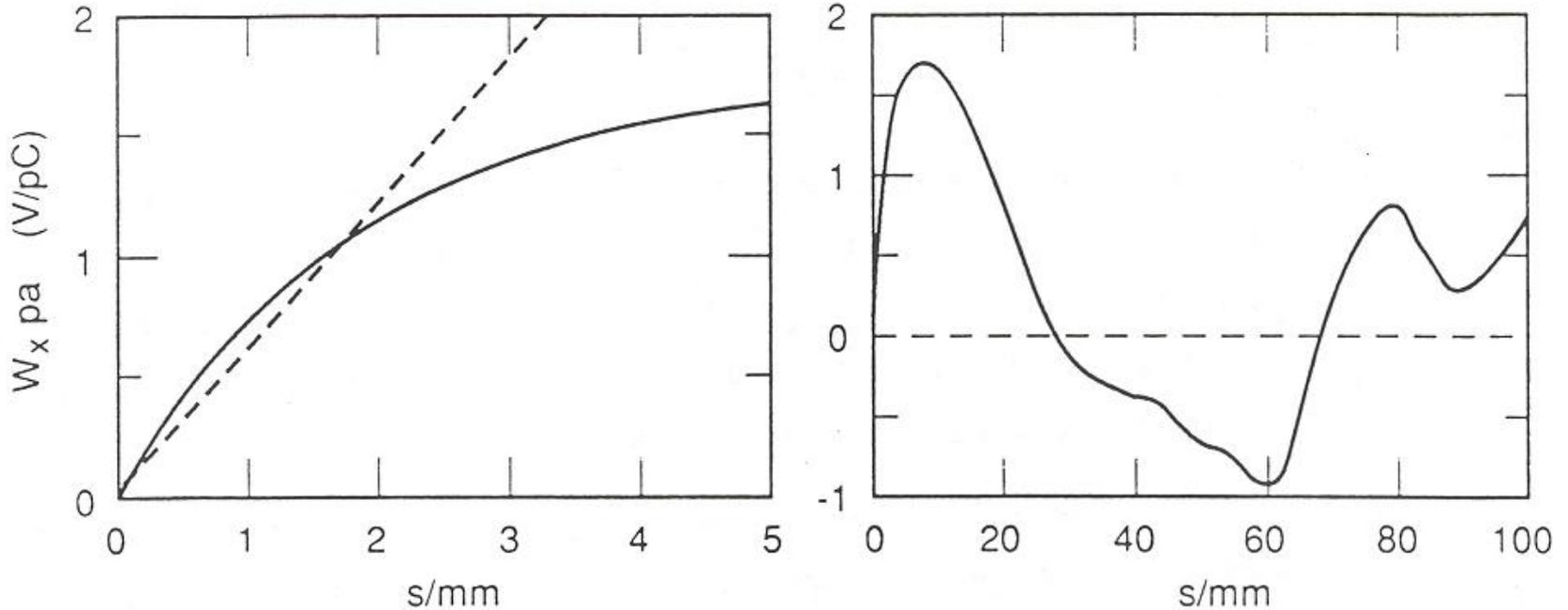
Fig. 9. Transverse wakefield per cell for the SLAC structure for a particle at the iris radius. The dashed line is a linear approximation to the wake seen by a 1 mm bunch.
