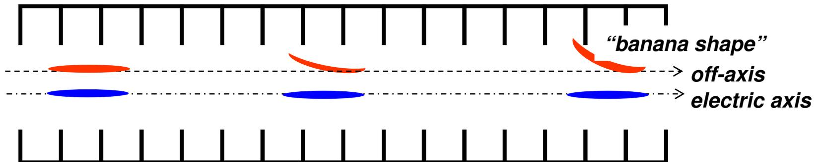
The induced transverse **projected emittance growth** can be counteracted by “damping” the trailing particles’ oscillation amplitude:
