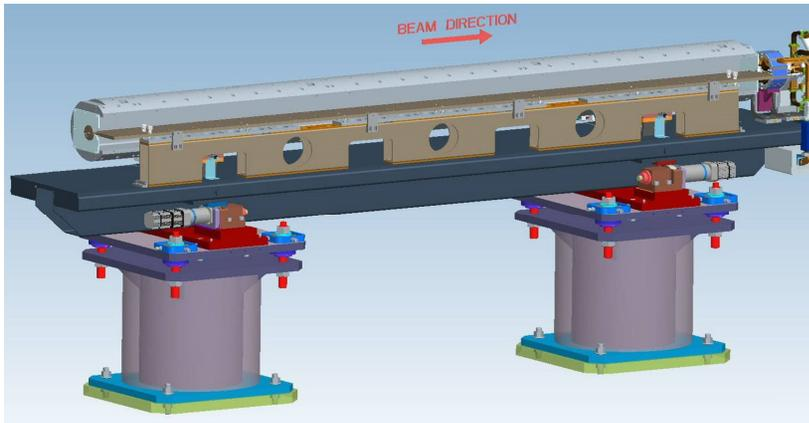
1. Use fixed, stable support (especially for RF structures) and girder with 3-D movers on the top of it.
