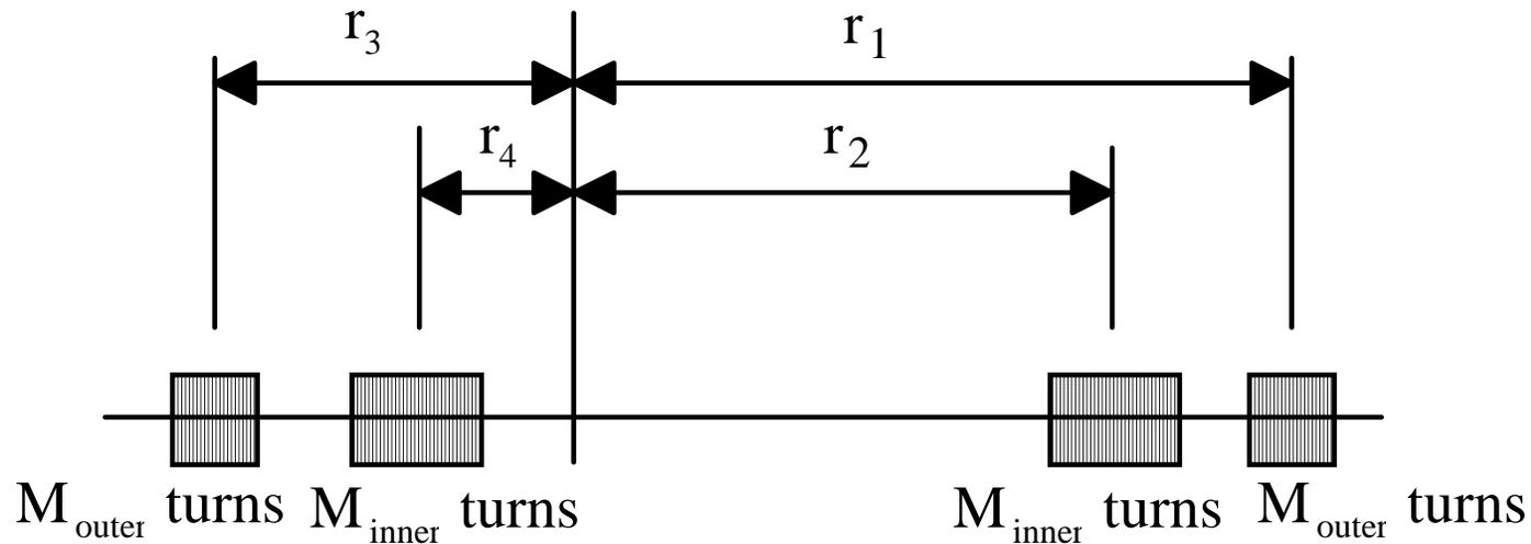
Two sets of nested coils with  $M_{outer}$  and  $M_{inner}$  number of turns to increase the output voltage for the outer and inner coils, respectively, are illustrated.
