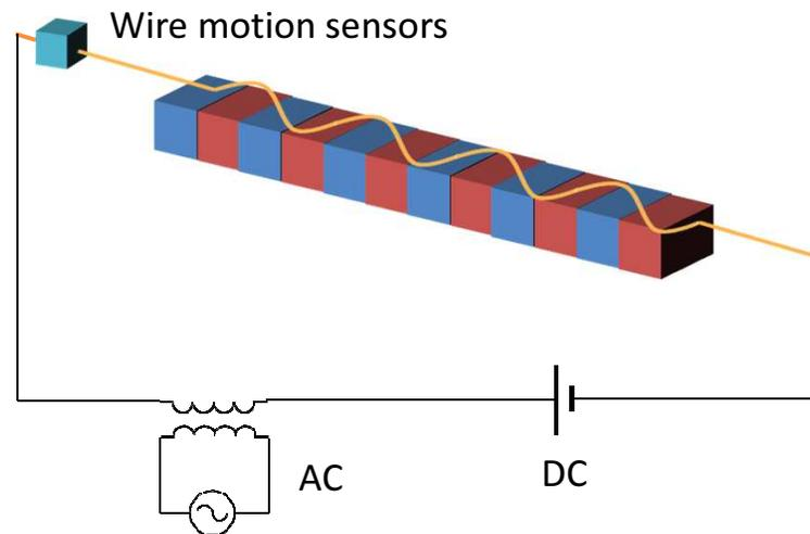
\* A. Temnykh, "VIBRATING WIRE AND FLIPPING COIL MAGNETIC MEASUREMENT OF A CESR-C 7-POLE WIGGLER MAGNET"
