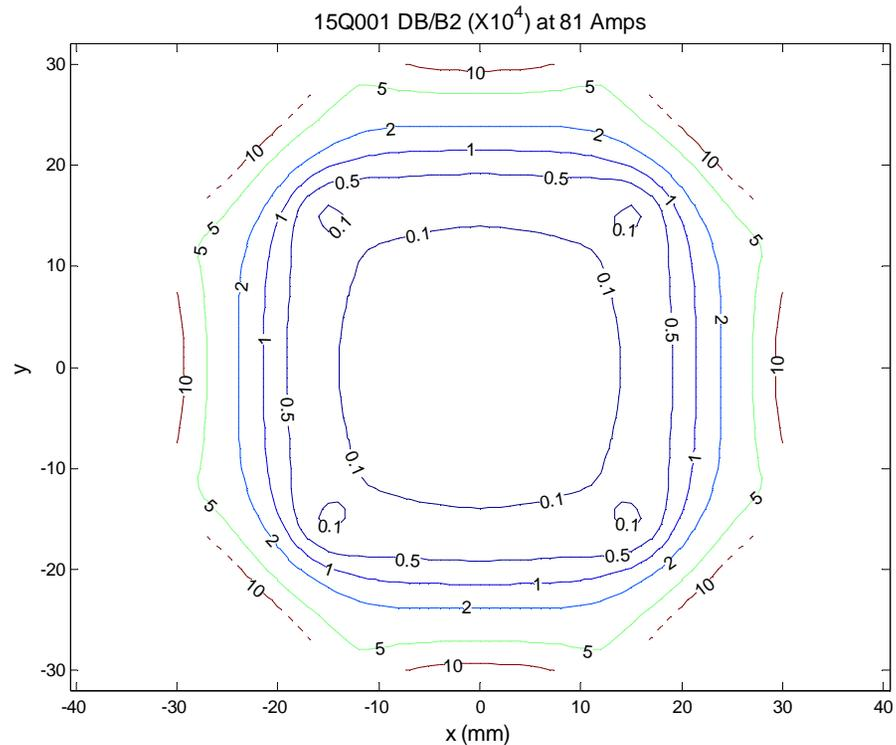
When the iso-error curve is replotted with the unallowed multipole errors reduced to zero and the allowed multipole phases adjusted to eliminate the skew terms, the  $\Delta B/B < 10^{-4}$  region is dramatically increased. This illustrates the importance of the first three unallowed multipole errors which are primarily the result of magnet fabrication and assembly errors.
