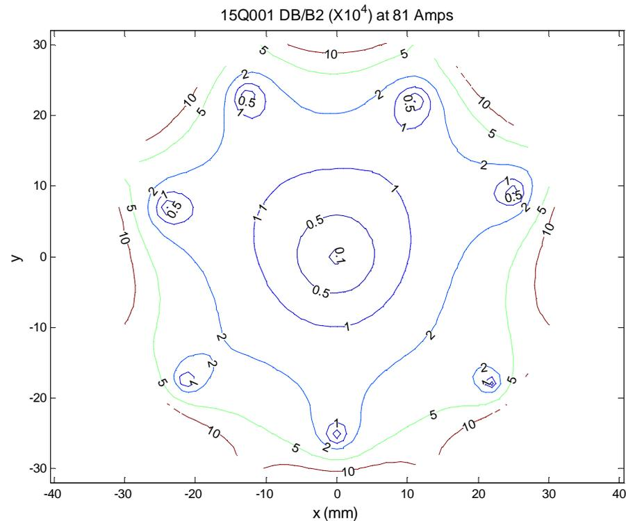
The iso-error plot is replotted for only the allowed multipoles ( $n=6, 10, 14$  and  $18$ ) and the first three unallowed multipoles ( $n=3, 4$  and  $5$ ). It can be seen that it is virtually identical with the previous plot, indicating that the unallowed multipole errors  $> 6$  are not important.
