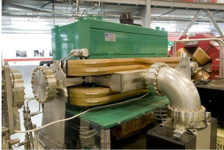
Sextupole magnets to focus off-energy electrons (mainly)
