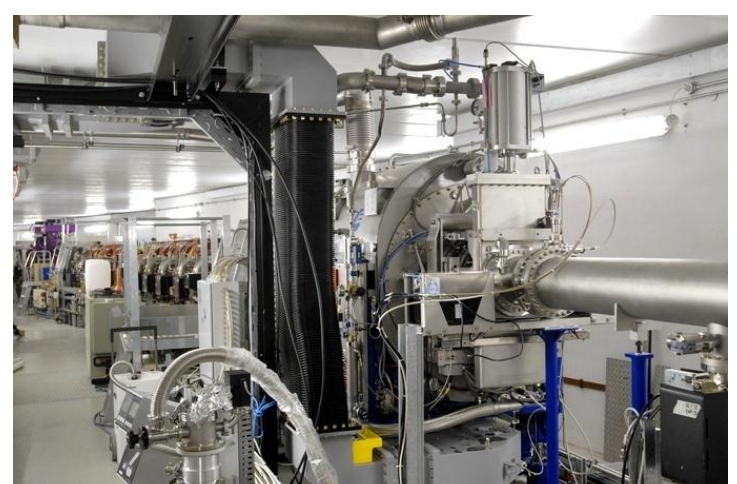
RF cavities to accelerate or replace E losses due to synchrotron radiation
