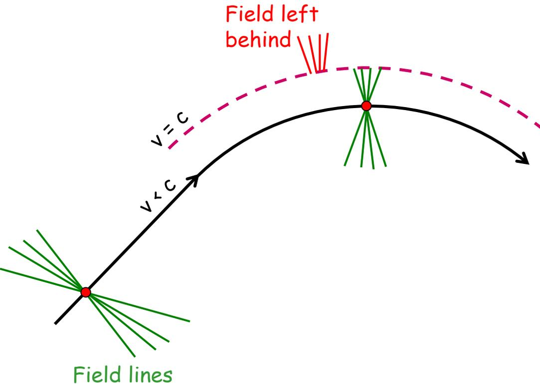
*Energy loss per meter is proportional to the energy in the 4th degree*
