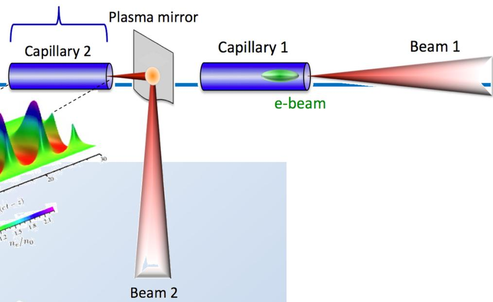
Concept of 1 TeV linear collider based on laser acceleration
